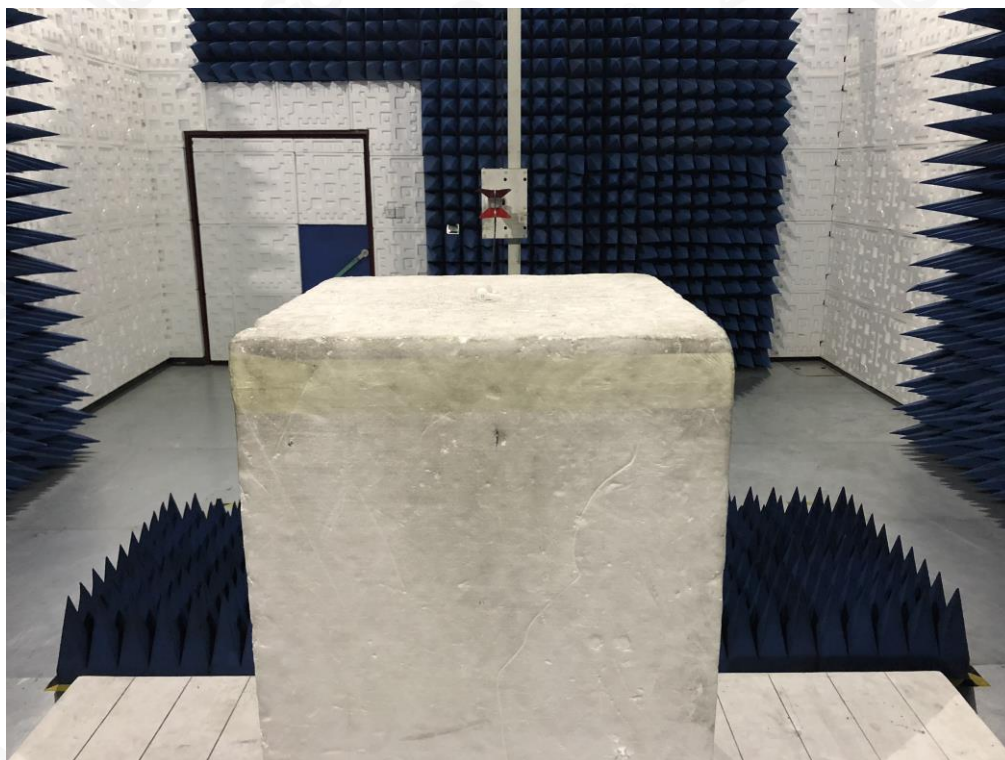
RADIATED EMISSION TEST SETUP ABOVE 1GHZ
