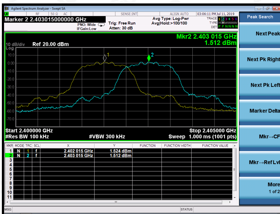
TEST PLOT FOR FREQUENCY SEPARATION
