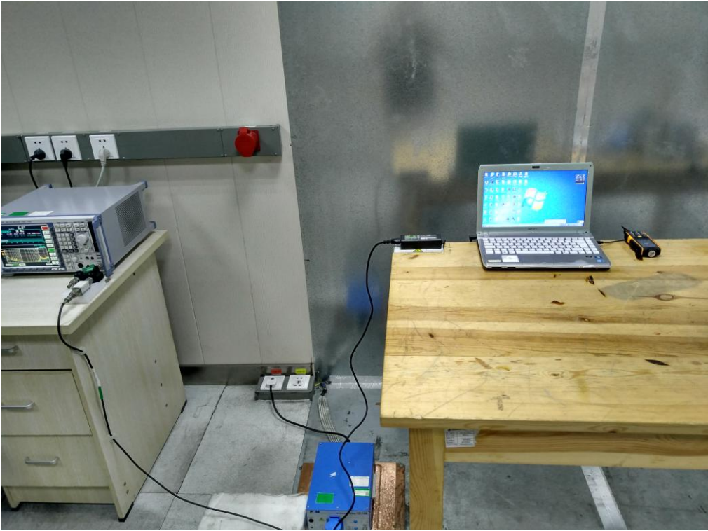
FCC RADIATED EMISSION TEST SETUP
