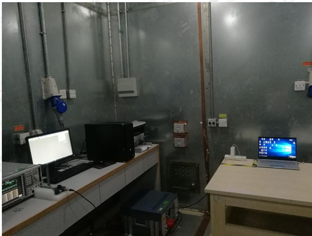
FCC RADIATED EMISSION TEST SETUP BELOW 1GHZ
