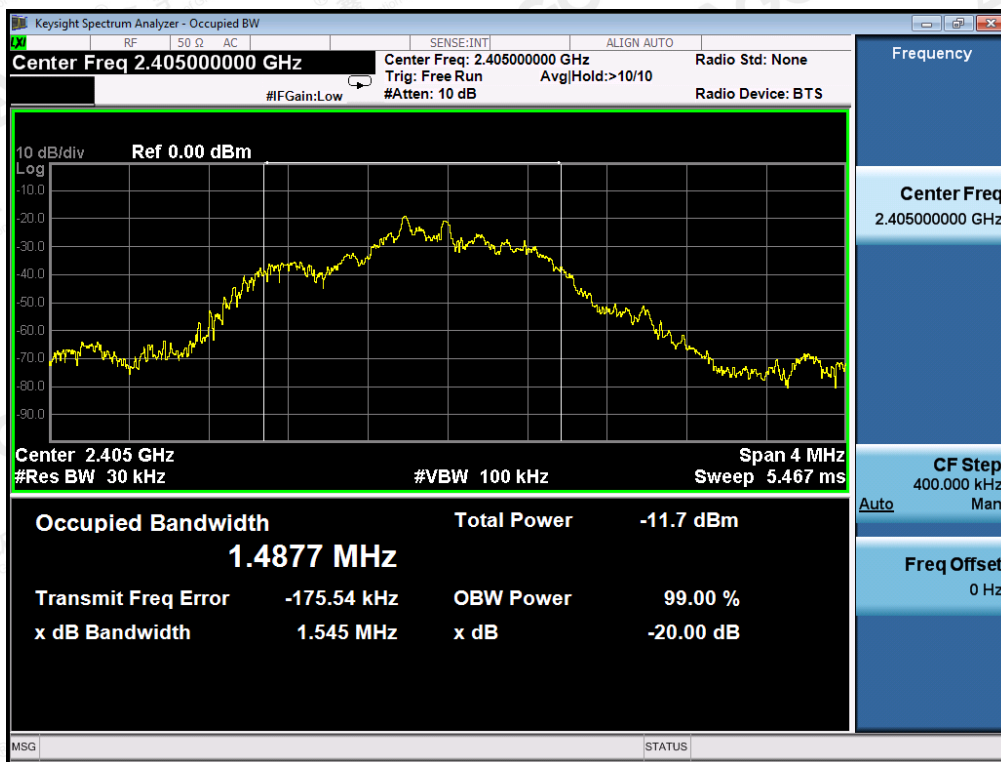
TEST PLOT OF BANDWIDTH FOR LOW CHANNEL
