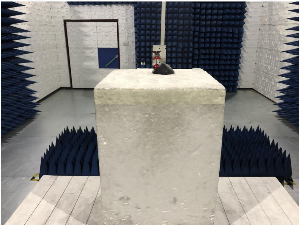
RADIATED EMISSION TEST SETUP ABOVE 1GHZ
