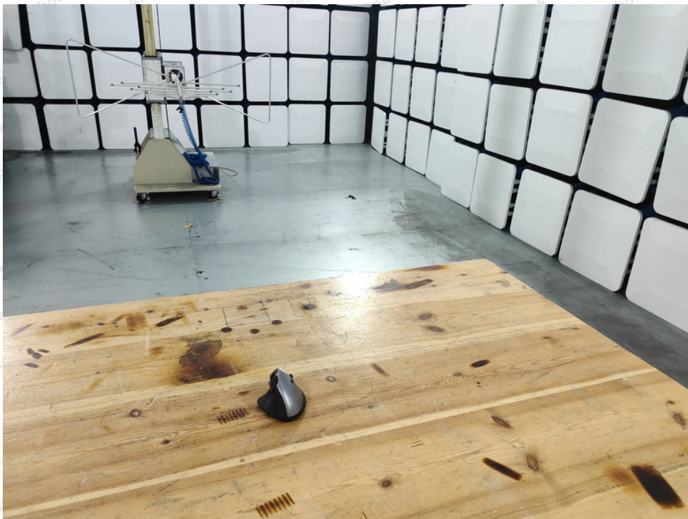
Photo of Radiation Emission Test
