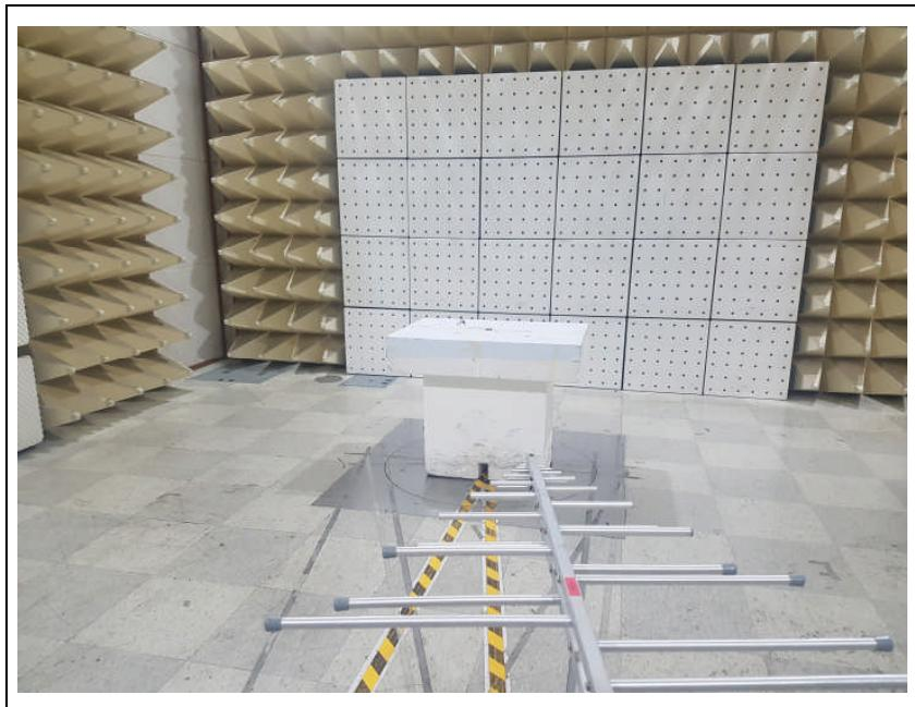
**B. Photo of Radiated Spurious Emission Test (Above 1 GHz)**
