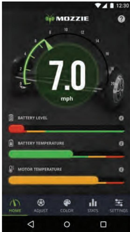
This screen allows you to track your current speed, the battery level and the temperature for the battery and motor. Utilize extreme caution and be aware of your surroundings while using the app. Always look in the direction you are moving as well as either side of you.
