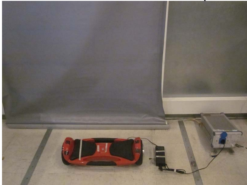
Measurement of Conducted Emission Test Set Up
