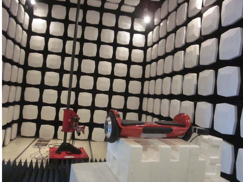
Measurement of Radiated Emission Test Set Up
