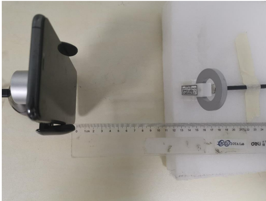
H-field Test Setup Photo Positon E (15cm)
