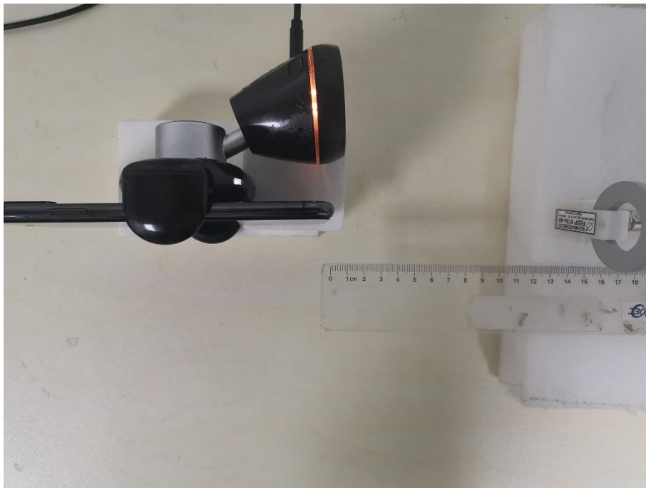
H-field Test Setup Photo Positon D (15cm)
