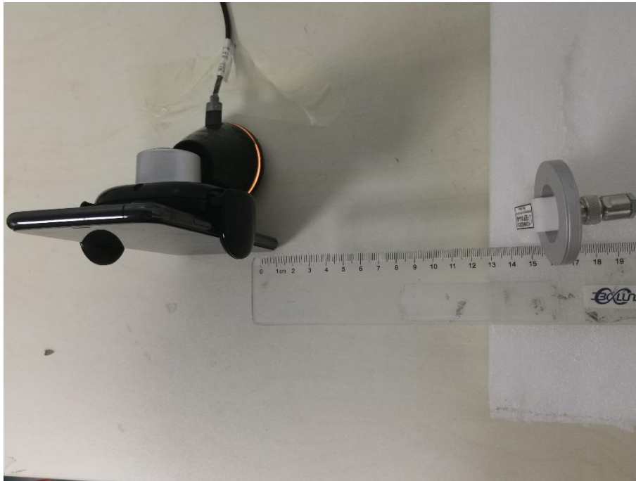
H-field Test Setup Photo Positon A (15cm)
