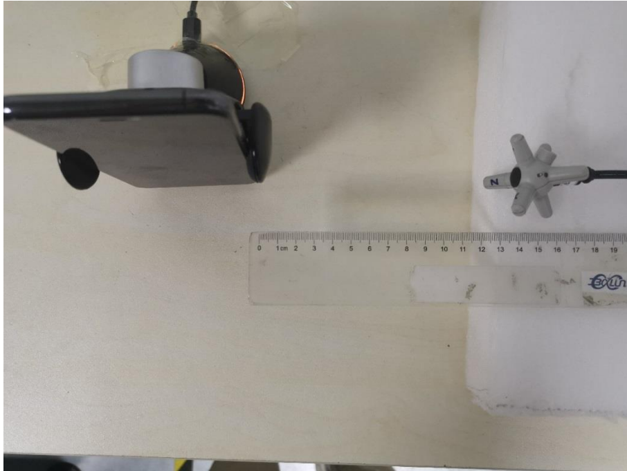
E-field Test Setup Photo Positon A (15cm)
