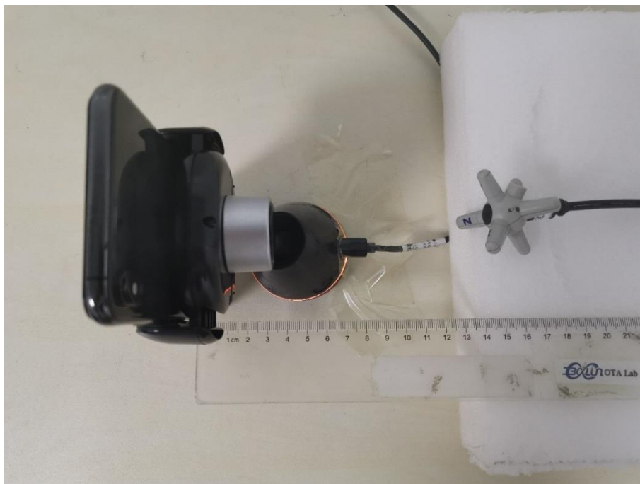
E-field Test Setup Photo Positon F (15cm)
