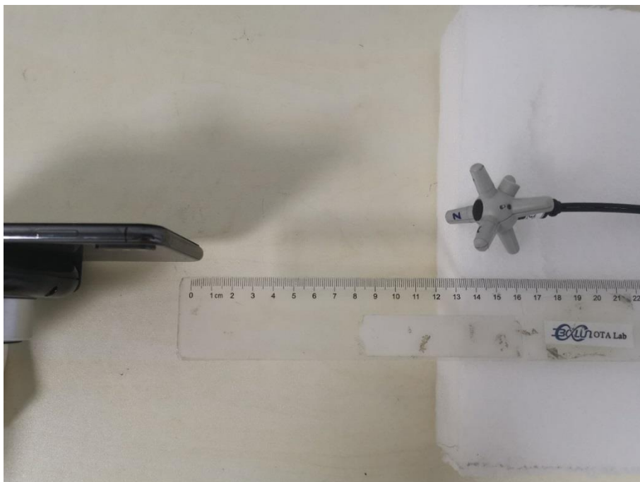
E-field Test Setup Photo Positon B (15cm)
