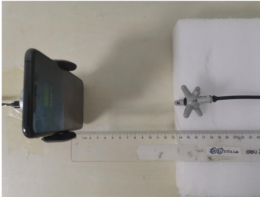
E-field Test Setup Photo Positon E (15cm)
