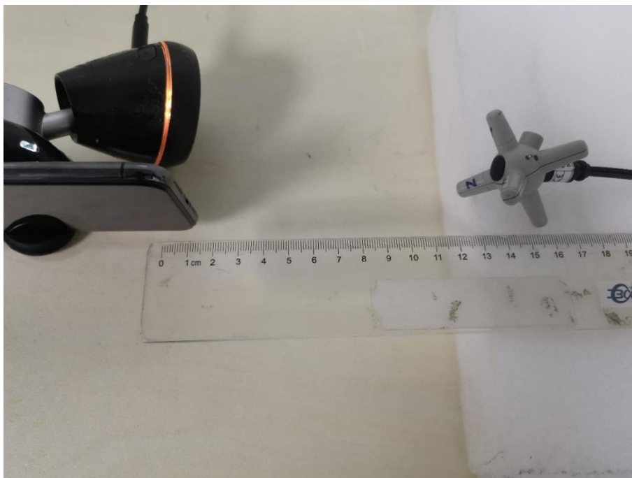
E-field Test Setup Photo Positon D (15cm)
