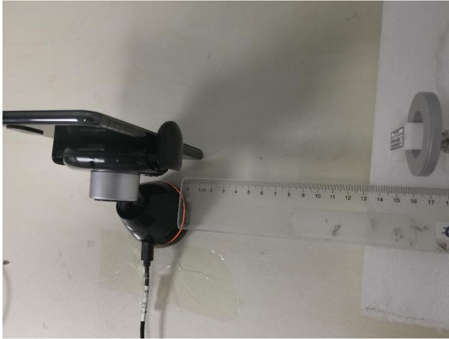
H-field Test Setup Photo Positon C (15cm)
