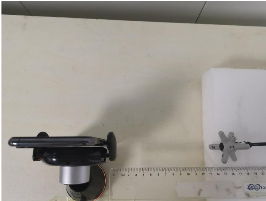
E-field Test Setup Photo Positon C (15cm)
