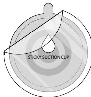
2. Peel off the protective film on the Suction Cup and press firmly onto the windshield.
