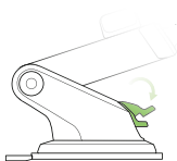
3. Push Locking Lever down to secure mount.
