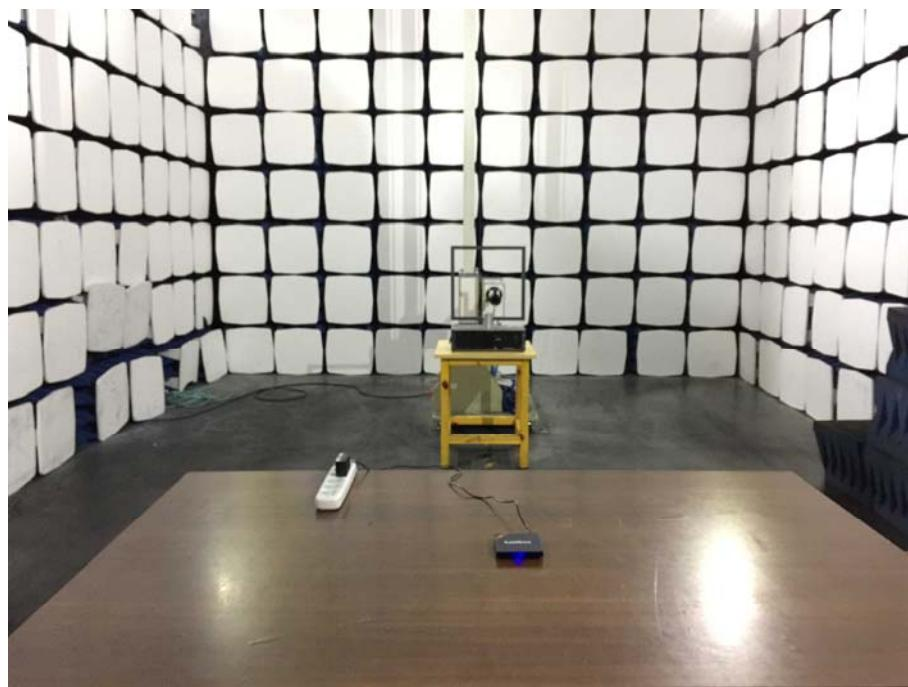
**Radiation Emission Test Setup (30MHz to 1GHz)**
