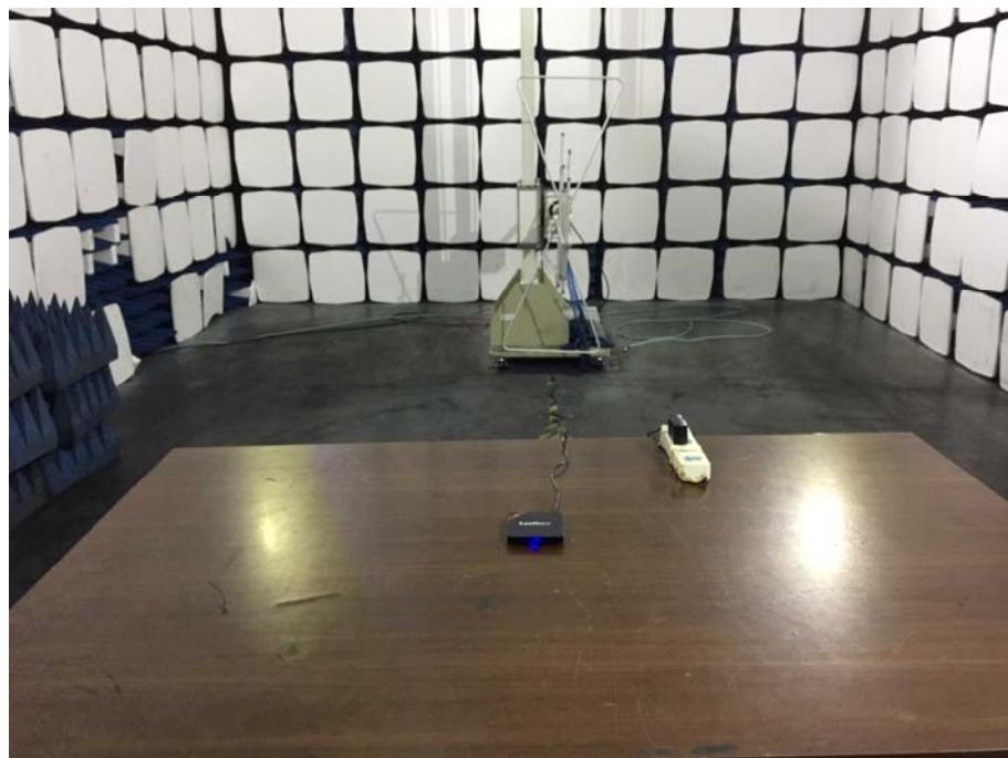
**Radiation Emission Test Setup (Above 1GHz)**
