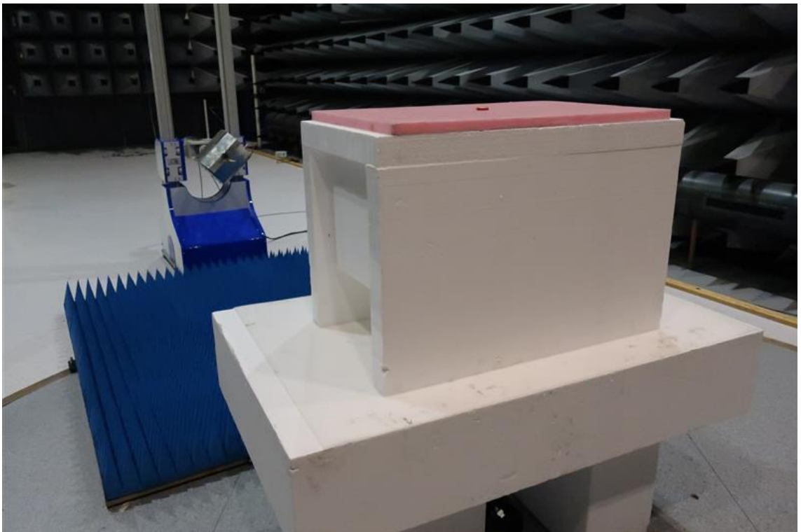
Photo 4.6.2 Test setup regarding measurement of field strength of fundamental.
