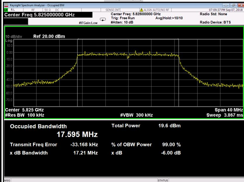
**IEEE 802.11n HT 20 MHz mode / 5745 ~ 5825MHz****6dB Bandwidth (CH Low)****Antenna 1**
