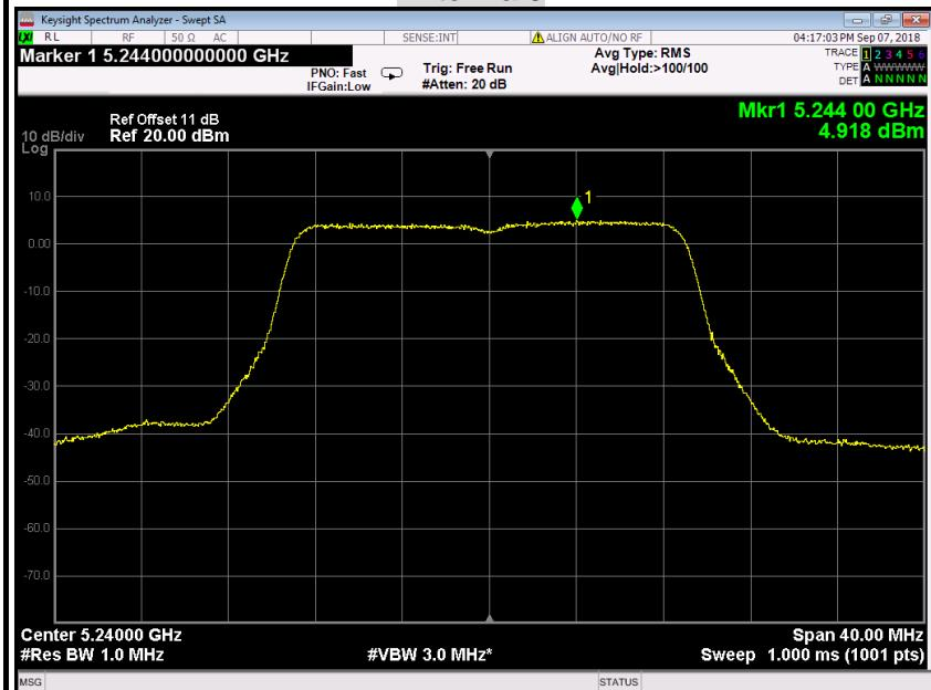
**IEEE 802.11n HT 20 MHz mode / 5745 ~ 5825MHz****PPSD (CH Low)****Antenna 0**
