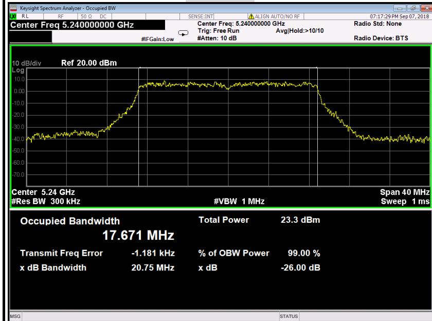
**IEEE 802.11n HT 20 MHz mode / 5180 ~ 5240MHz****26dB Bandwidth (CH Low)****Antenna 1**
