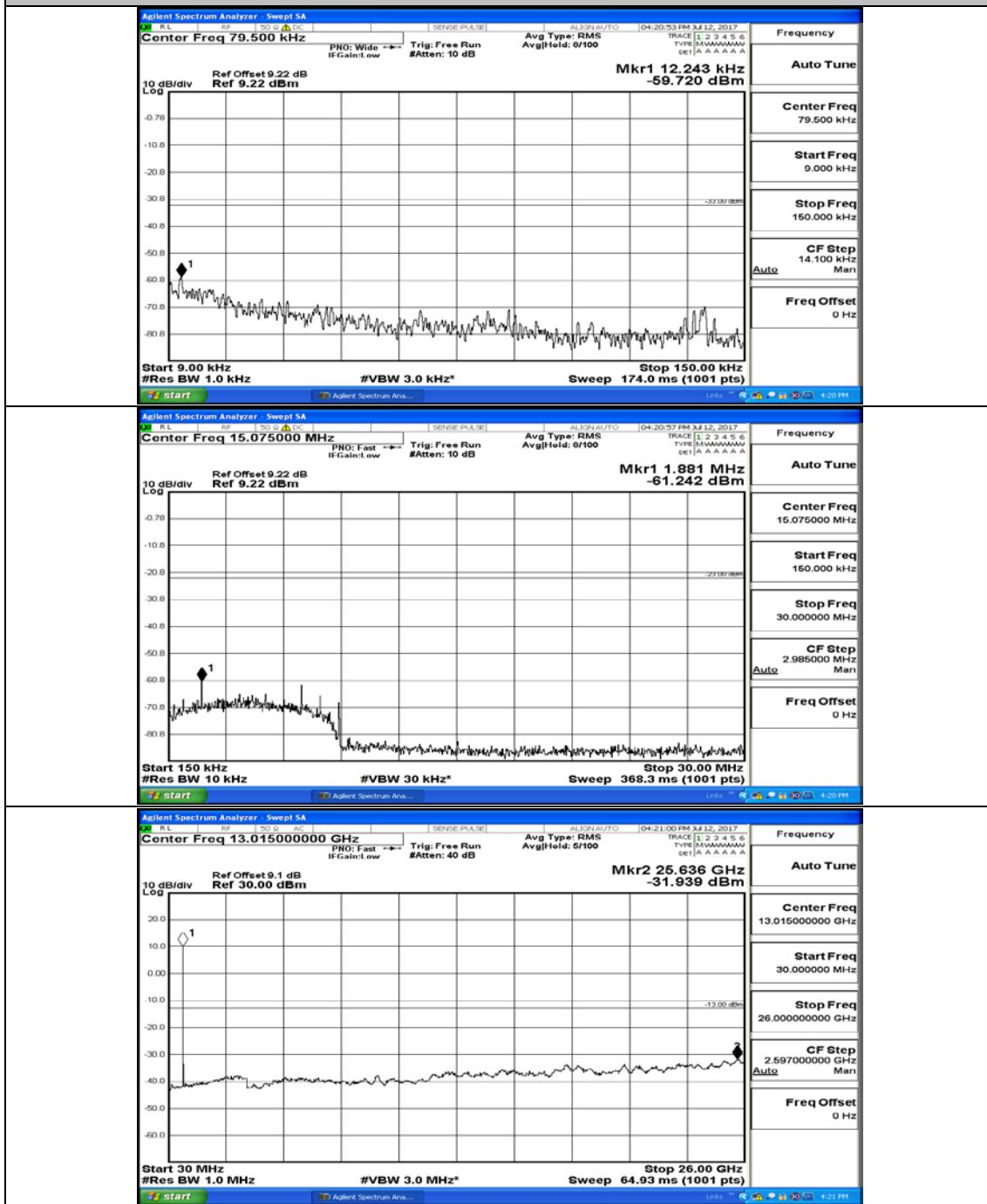
Channel Bandwidth: 10 MHz\_HCH\_QPSK\_50RB#0
