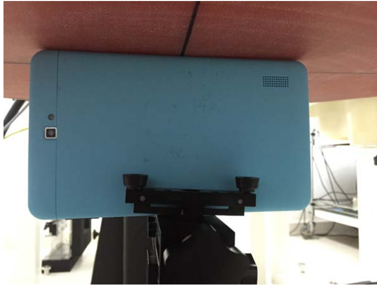
Test Position 3 - Body-worn, the right side of the EUT towards ground (The distance was 0mm)
