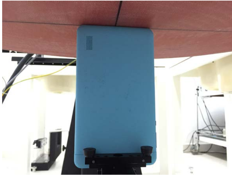
Test Position 5 - Body-worn, the bottom side of the EUT towards ground (The distance was 0mm)
