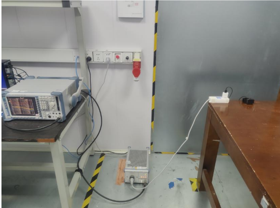
Conducted emissions at AC power line (150kHz-30MHz)
