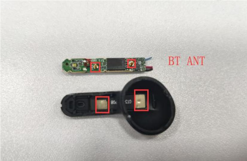
The photograph shows the internal antenna assembly. At the top, a green printed circuit board (PCB) is visible with two red squares highlighting specific connection points. Below the PCB is a black circular component, likely a connector or housing, with two small gold-colored rectangular pads. Red squares are also placed over these pads. The text "BT ANT" is written in red in the upper right area of the image.
