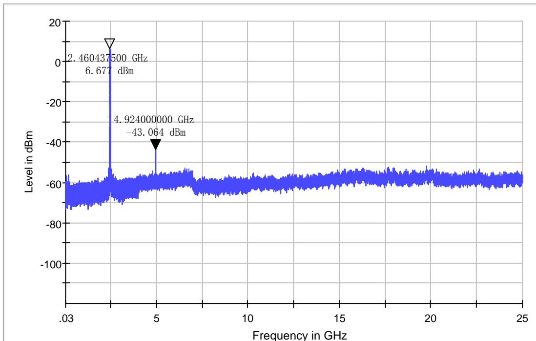
In any 100kHz bandwidth, the Conducted Spurious Emissions from 30 MHz to 25 GHz were greater than 20dB below the peak emission within the band that contains the highest level of the desired power.
