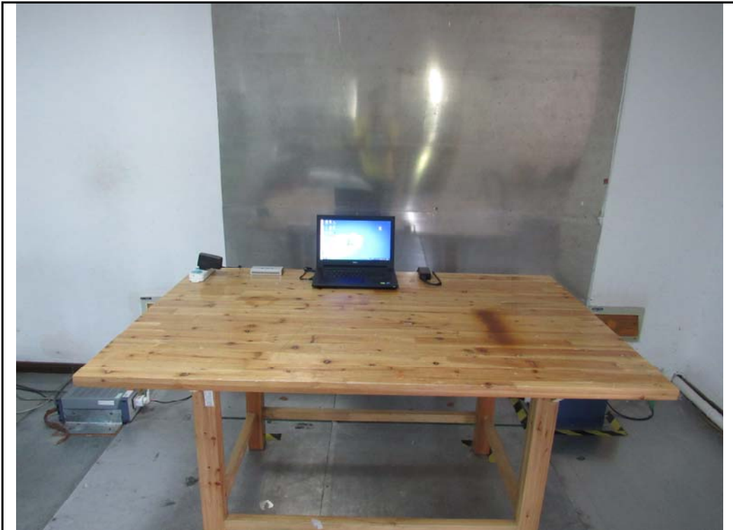
Conducted Emissions Test Setup Front View
