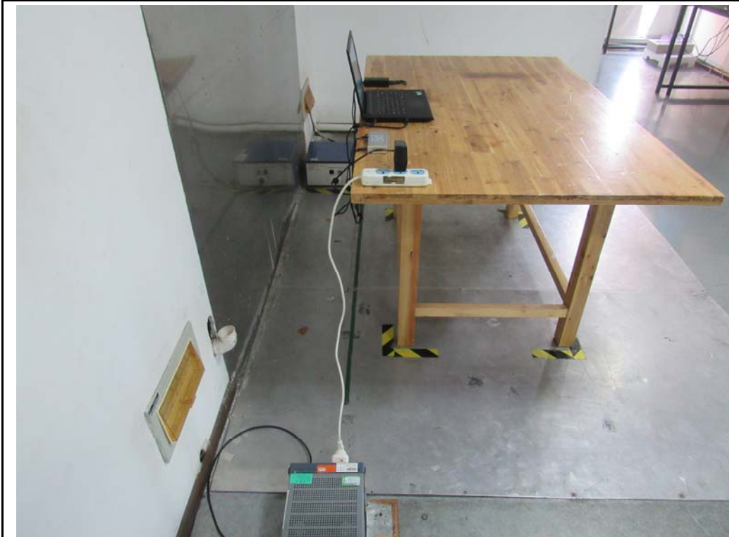
Conducted Emissions Test Setup Side View
