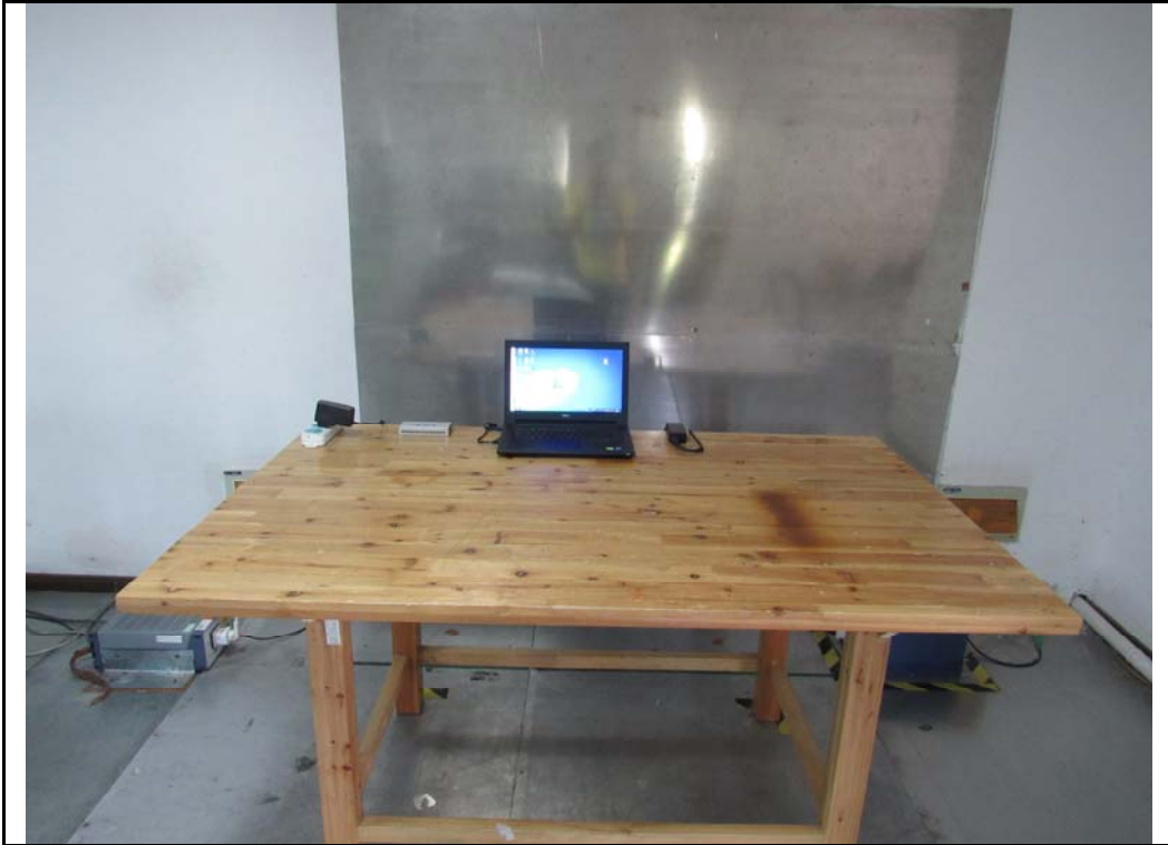
Conducted Emissions Test Setup Front View
