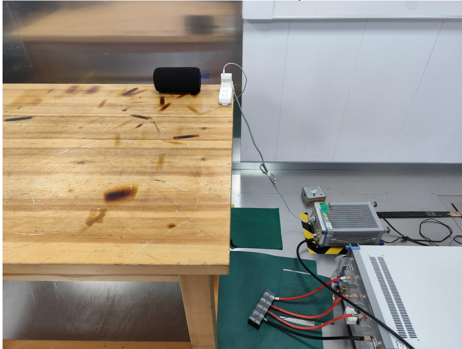
Conducted Emission at AC power line
