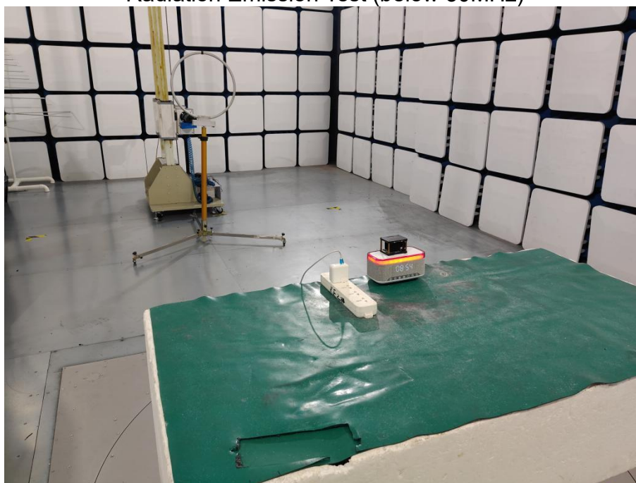
Radiation Emission Test (below 30MHz)
