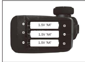
2. Assemble 3 pieces of 1.5V AA non-rechargeable batteries according to the polarity
