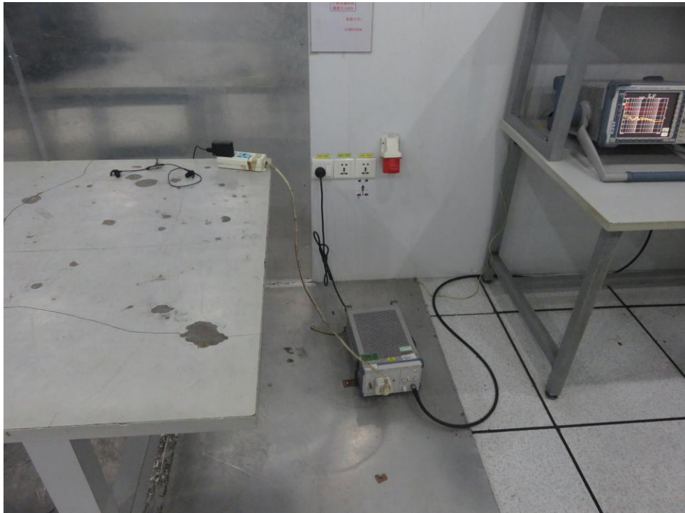
Photo of Conducted Emission Measurement
