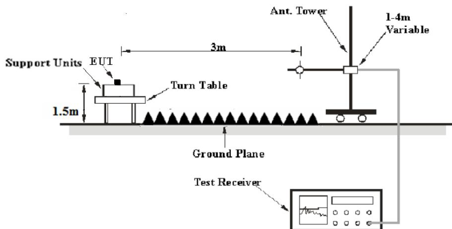
The radiated emission and out of band emission tests were performed in the 3 meters chamber test site, using the setup accordance with the ANSI C63.10-2013. The specification used was the FCC 15.209/15.205 and FCC 15.245 limits.
