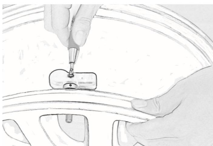
Step 2: Fix the sensor on the air nozzles with the sensor fixing screw. Note that the sensor should be close to the hub with a torque of  $4\text{N}\cdot\text{m}$ .
