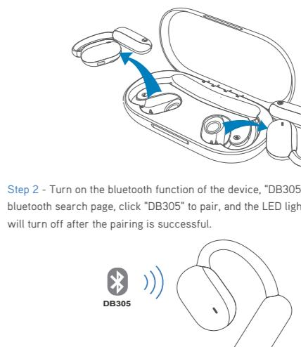
**Step 2:** Turn on the bluetooth function of the device, "DB305" will appear on the bluetooth search page, click "DB305" to pair, and the LED light of the earphones will turn off after the pairing is successful.
