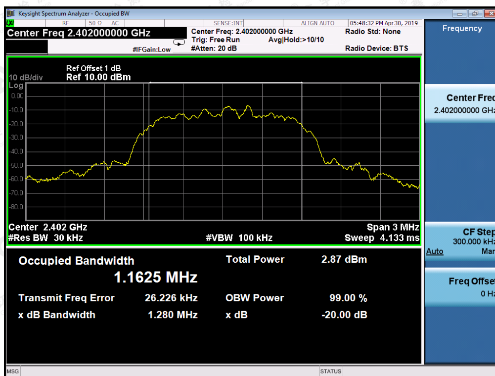
TEST PLOT OF BANDWIDTH FOR LOW CHANNEL
