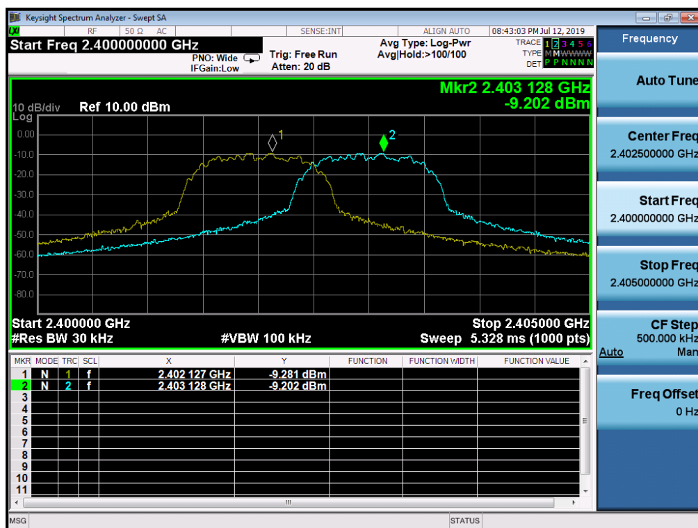
TEST PLOT FOR FREQUENCY SEPARATION
