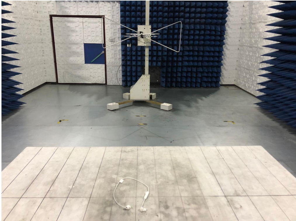
RADIATED EMISSION TEST SETUP ABOVE 1GHZ
