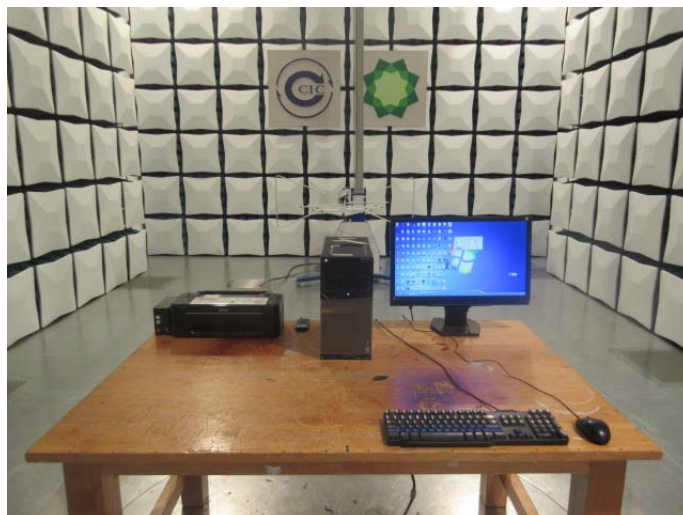
Radiated Emission (above 1GHz) Connect to PC
