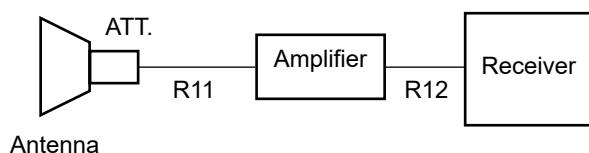
Diagram of the measurement instruments (Above 18 GHz)
