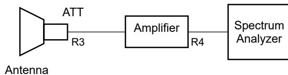
Diagram of the measurement instruments ( 1000- 2000 and 3000 – 18000 MHz)
