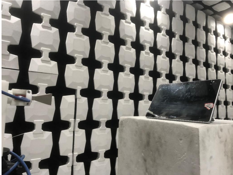
Description: Radiated Emission Test Setup (Above 18GHz)
