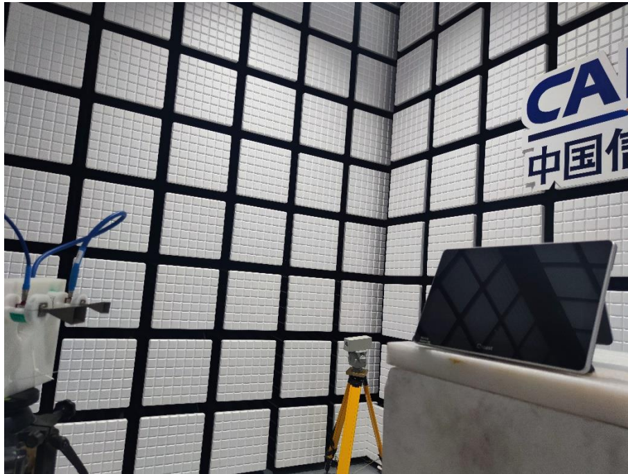
Description: Radiated Emission Test Setup (Above 18GHz)
