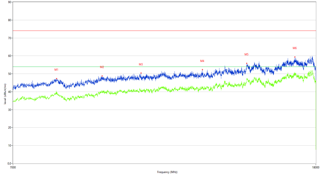
REmission Test case_FCC_Part 15C_FCC 15.247_7GHz-18GHz
