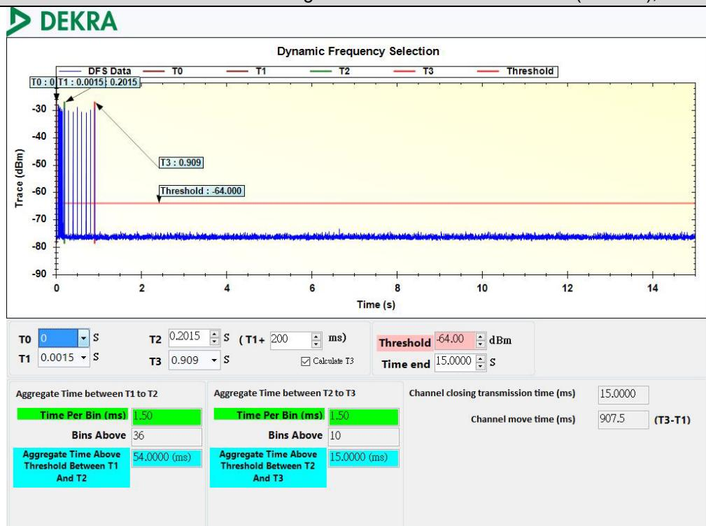
**Channel Move Time and Channel Closing Transmission Time - 802.11ax (40 MHz), 5510 MHz**
