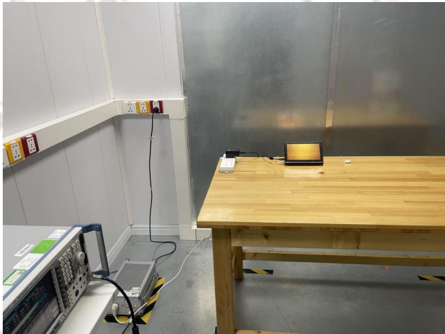
Radiated Emissions for 30MHz~1GHz
