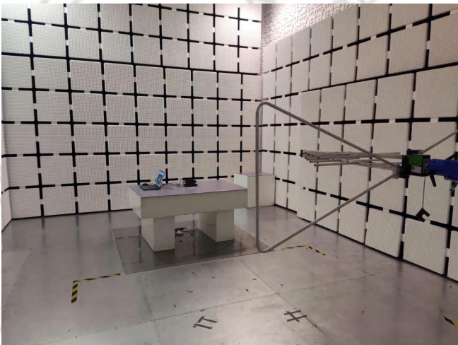
Radiated Emissions for above 18GHz
