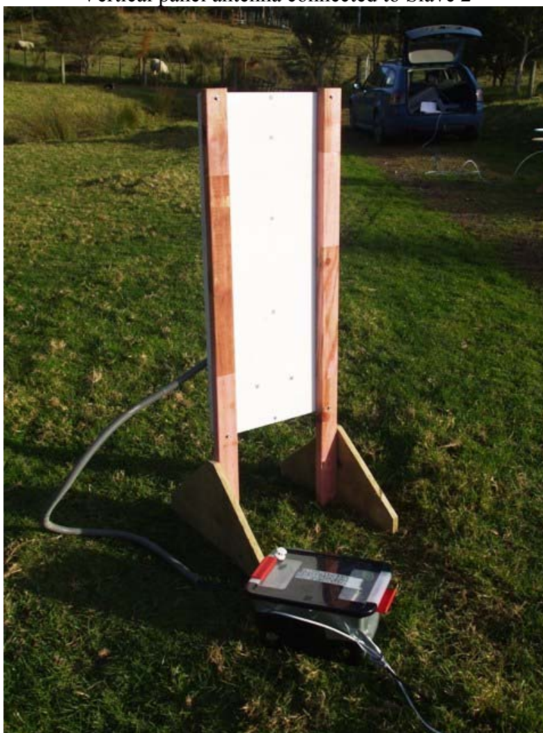
Vertical panel antenna connected to Slave 2
