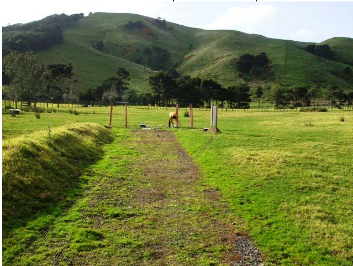
30 metre radiated emission test set up below 30 MHz. Loop antenna vertical
