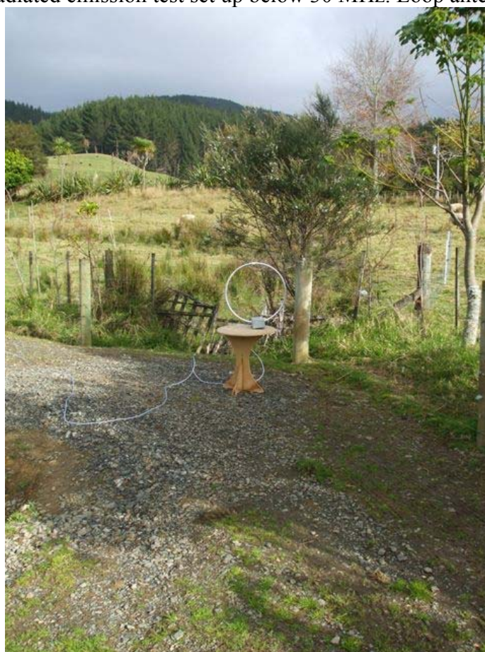
30 metre radiated emission test set up below 30 MHz. Loop antenna vertical
