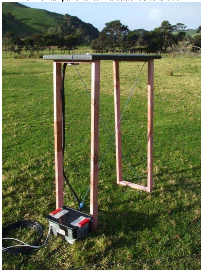
Horizontal panel antenna attached to Slave 1
