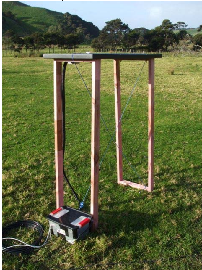
Horizontal panel antenna attached to Slave 1
