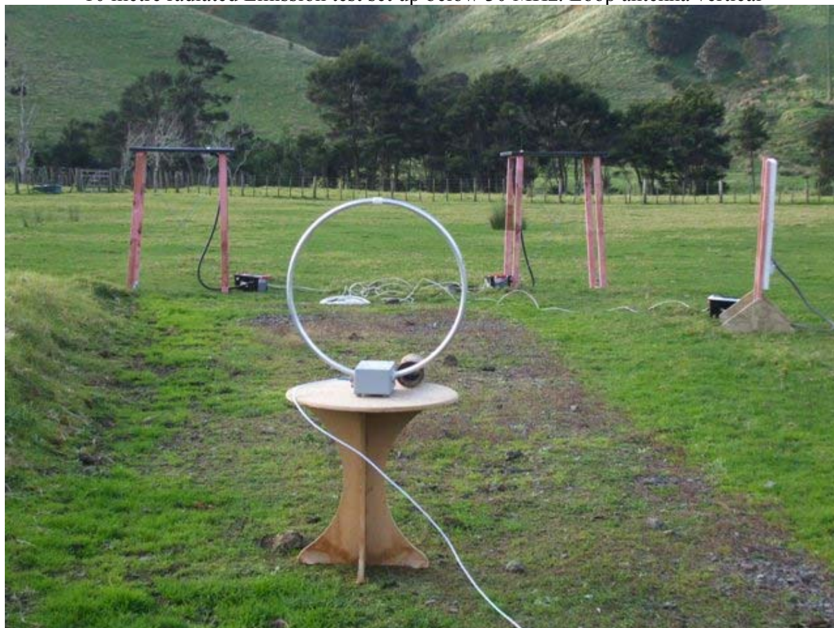
10 metre radiated Emission test set up below 30 MHz. Loop antenna vertical
