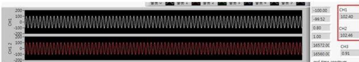
Figure 2.2 Result of amplitude accuracy measurement for brainwave signal channel. The measurement values were 102.4uVp and 102.5uV, respectively.
