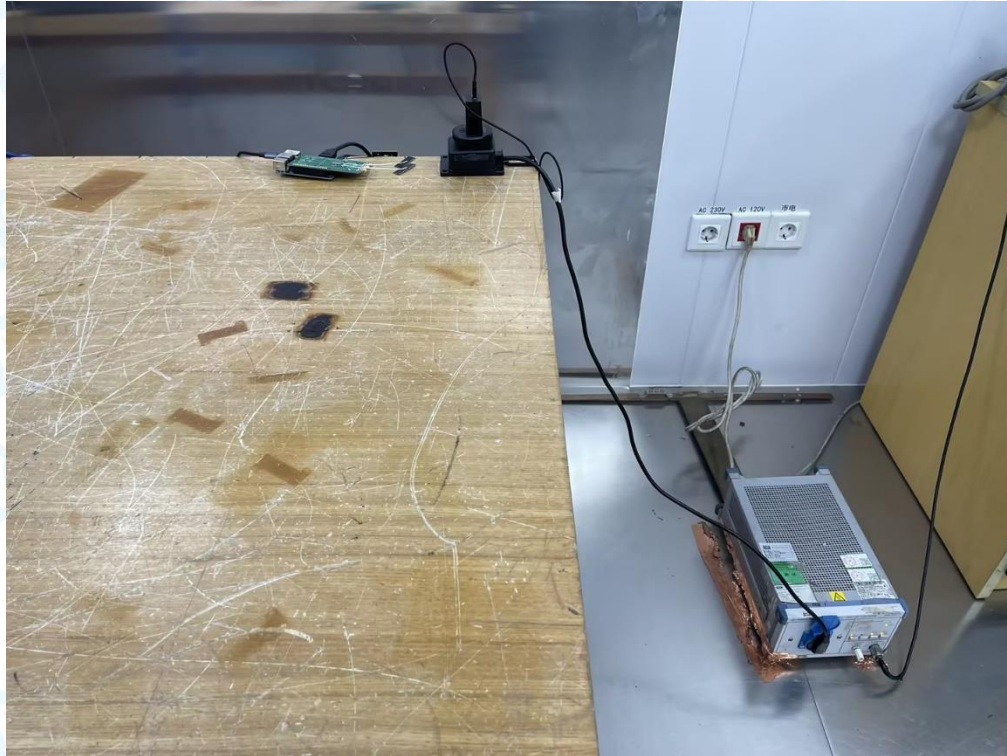
Photo of Setup for Radiated Emission (30MHz~1GHz)
