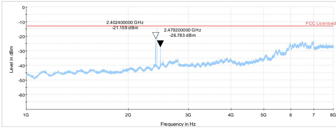
Peak above the limit is the uplink carrier frequency.
