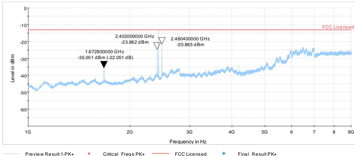
Peak above the limit is the uplink carrier frequency.
