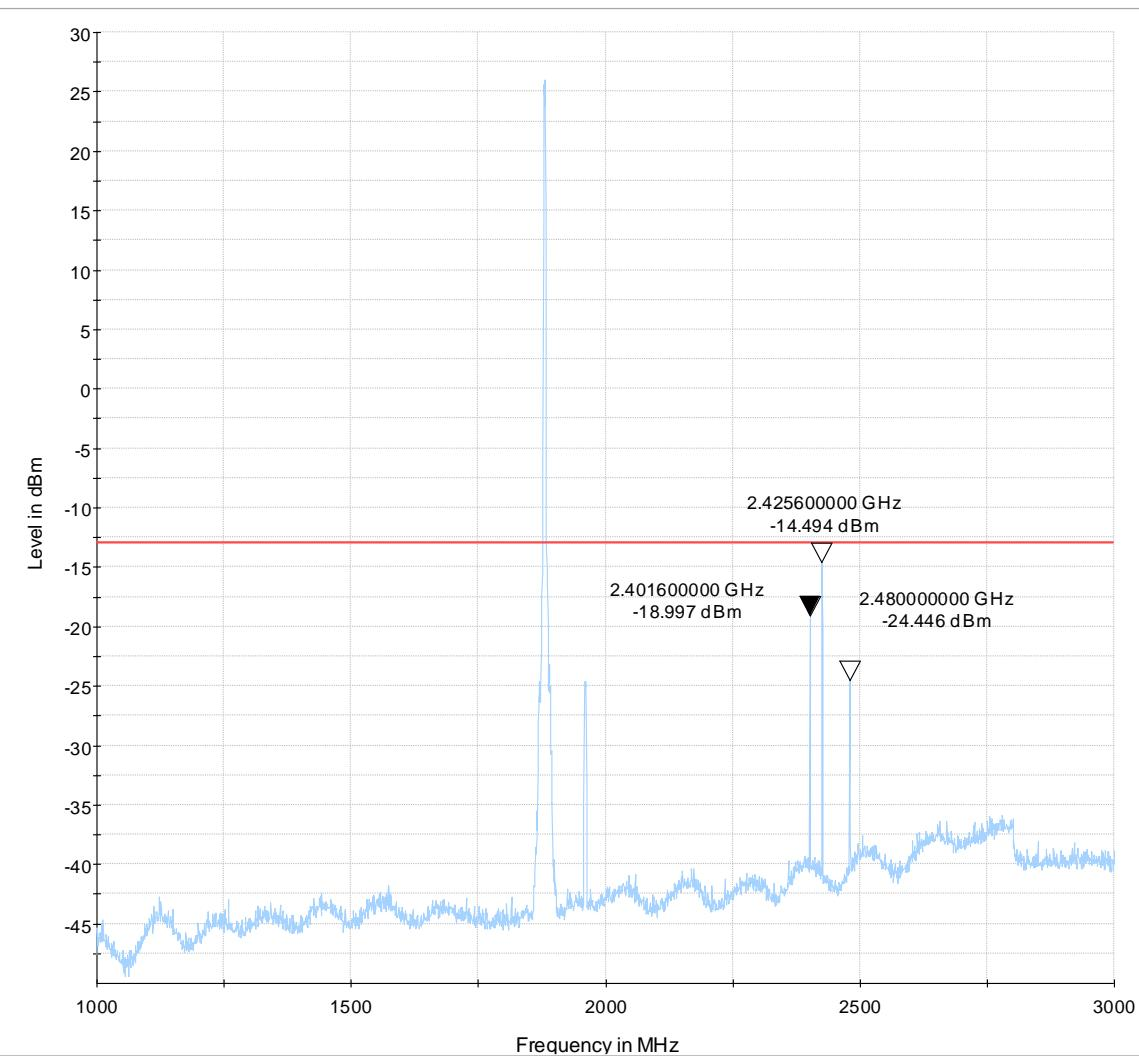
Peak above the limit is the uplink carrier frequency
