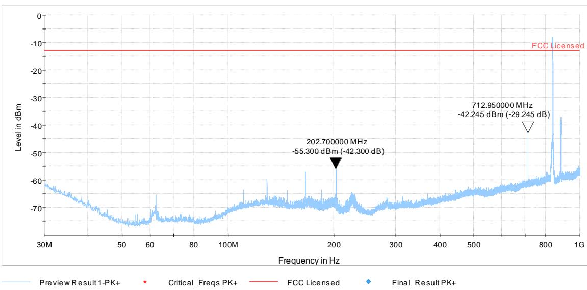
Peak above the limit is the uplink carrier frequency.
