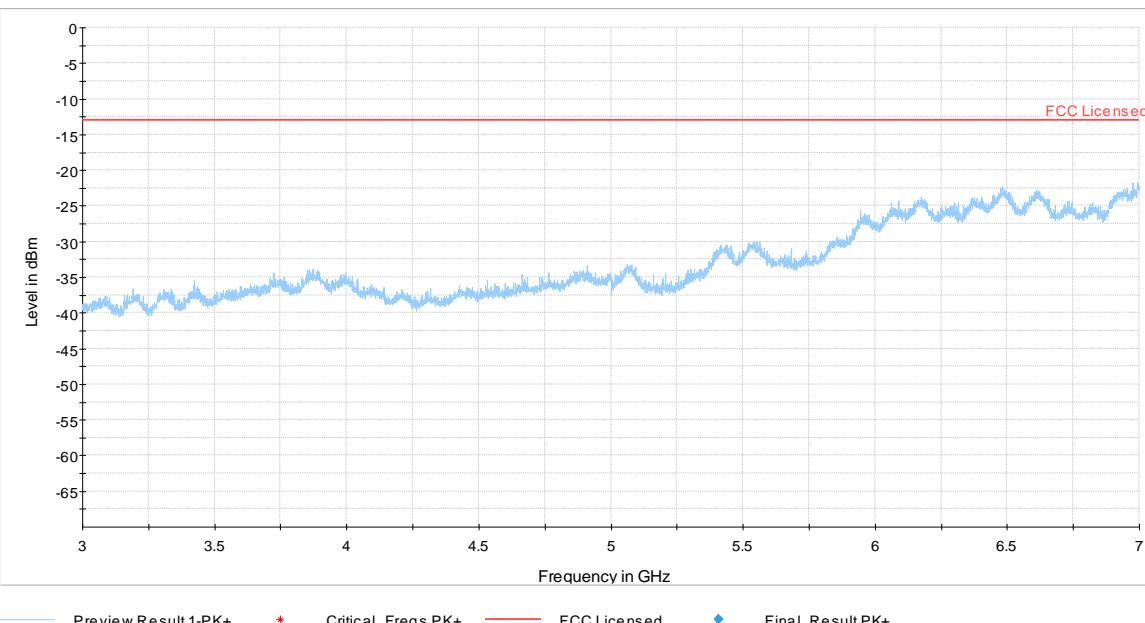
Peak above the limit is the uplink carrier frequency.
