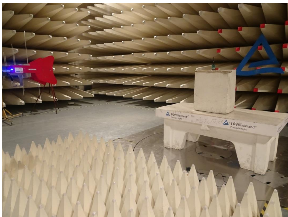
Horizontal Polarization Setup Photo - 18 GHz – 26.5 GHz
