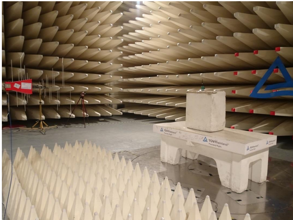
Vertical Polarization Setup Photo - 1 GHz – 18 GHz
