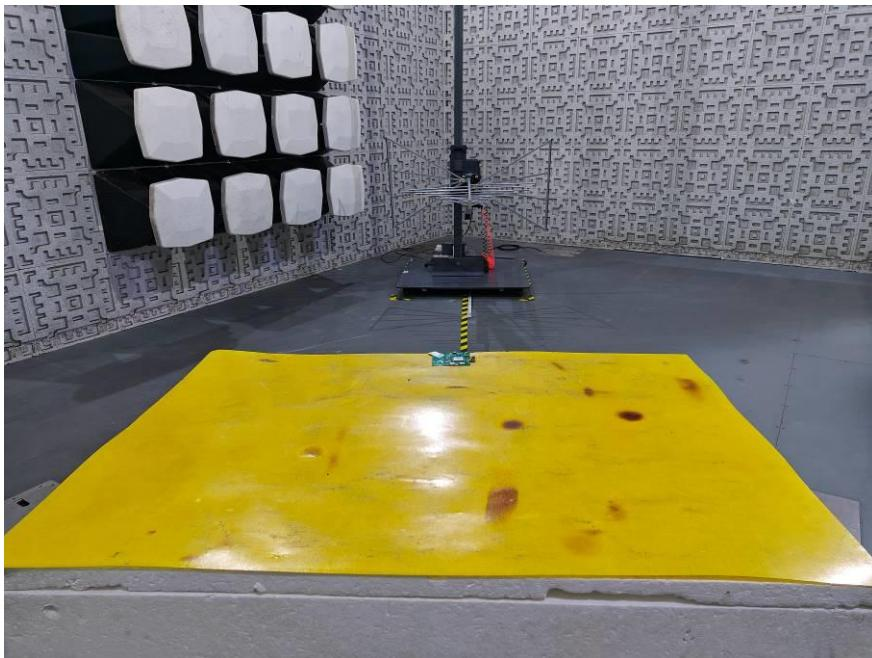
Spurious emissions at antenna terminals (Above 1GHz)
