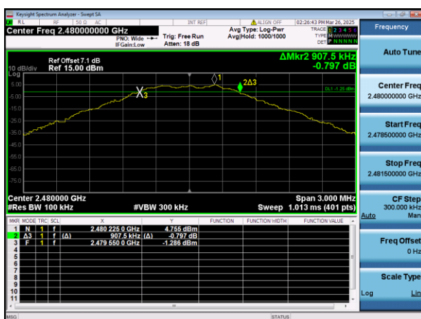
GFSK (BLE 1Mbps) HIGH CHANNEL
