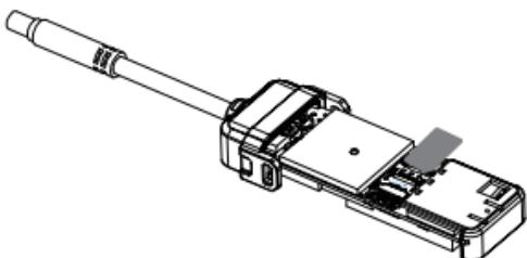
Insert SIM card into the slot and toggle the switch to ON
