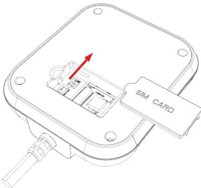
4. Lock the SIM card holder cover and secure the SIM card compartment cover.
