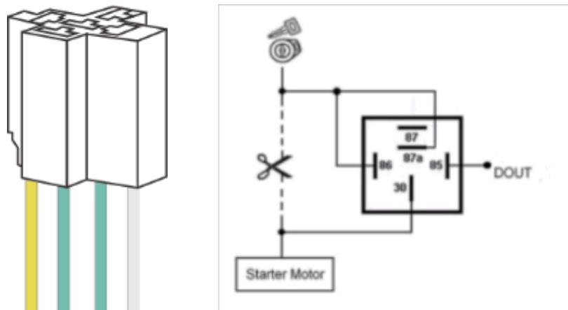
12V relay is standard. The device is suitable for vehicles with 12V supply. If the vehicle power supply is 24V, use 24V relay.
