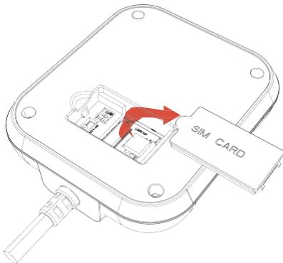
3. Insert SIM card into the slot and toggle the switch to ON.
