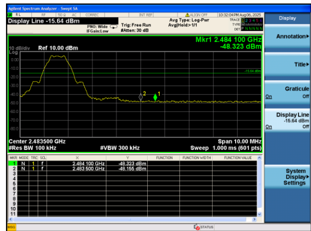
GFSK (BLE 1Mbps) HIGH CHANNEL, BAND EDGE
