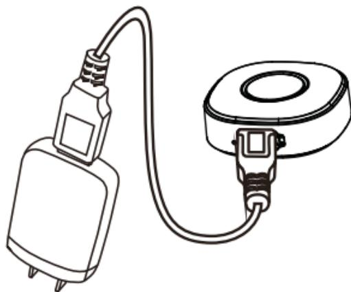
**Note:** It takes about 2.5 hours to fully charge the battery. It is normal that the device goes hot during charging.
