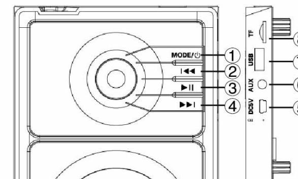
1.MODE : Long Press is power on-off function. Short press is mode shift (USB/TF, Bluetooth, LINE, FM etc.)
