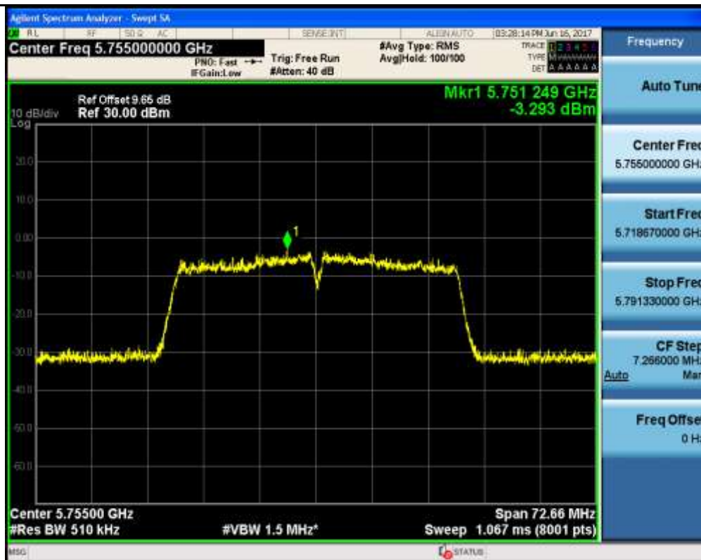
Maximum Conduct Output Power_TNVN_11AC40_5795_Ant1
