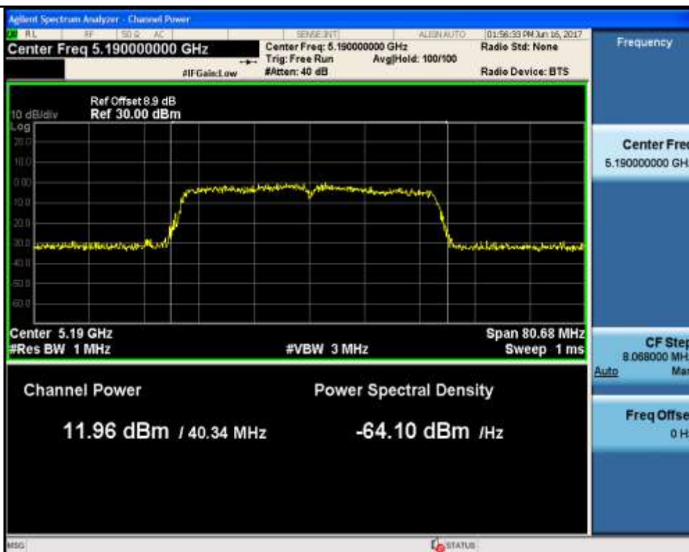
Maximum Conduct Output Power_11AC40_5230_Ant1
