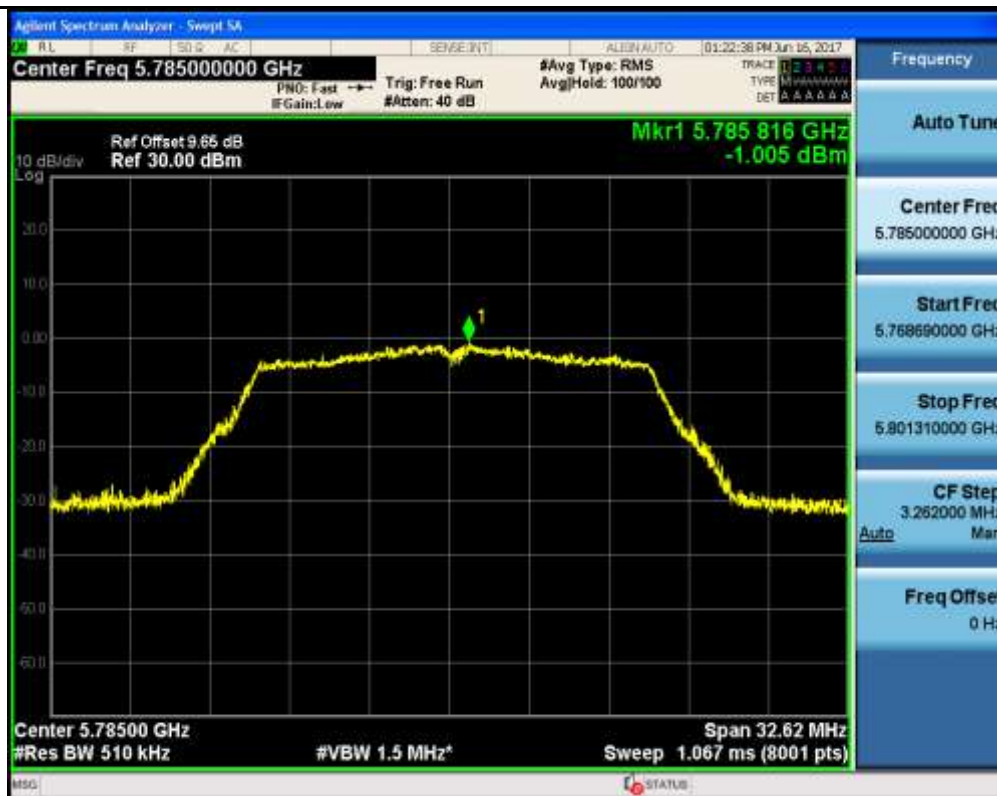
Maximum Conduct Output Power_TNVN_11A_5825_Ant1
