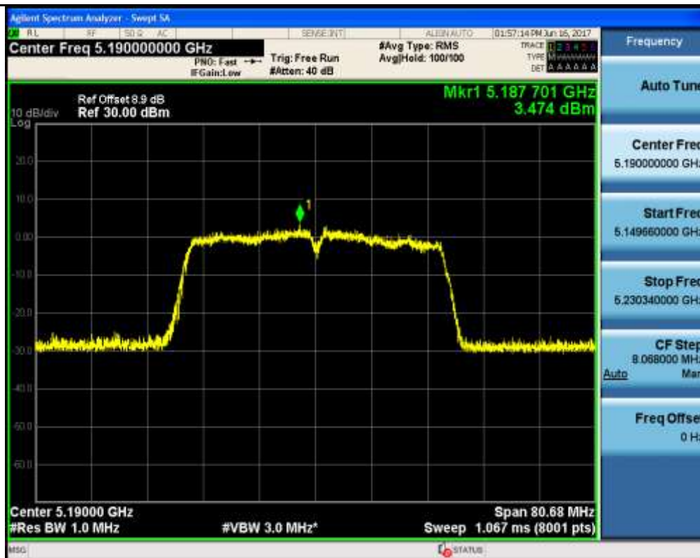
Maximum Conduct Output Power_TNVN_11AC40_5230_Ant1
