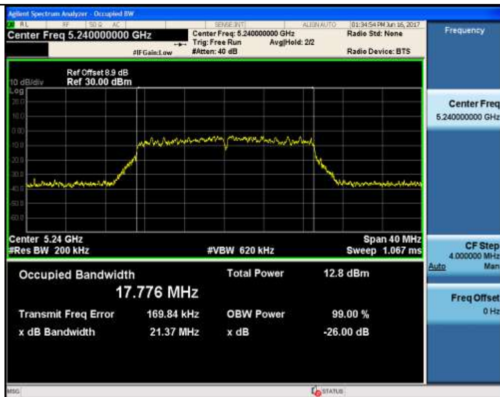
Emission Bandwidth Measurement_11AC20_5745_Ant1
