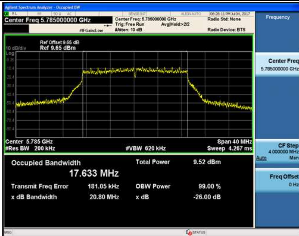
Emission Bandwidth Measurement_11AC20_5825_Ant1
