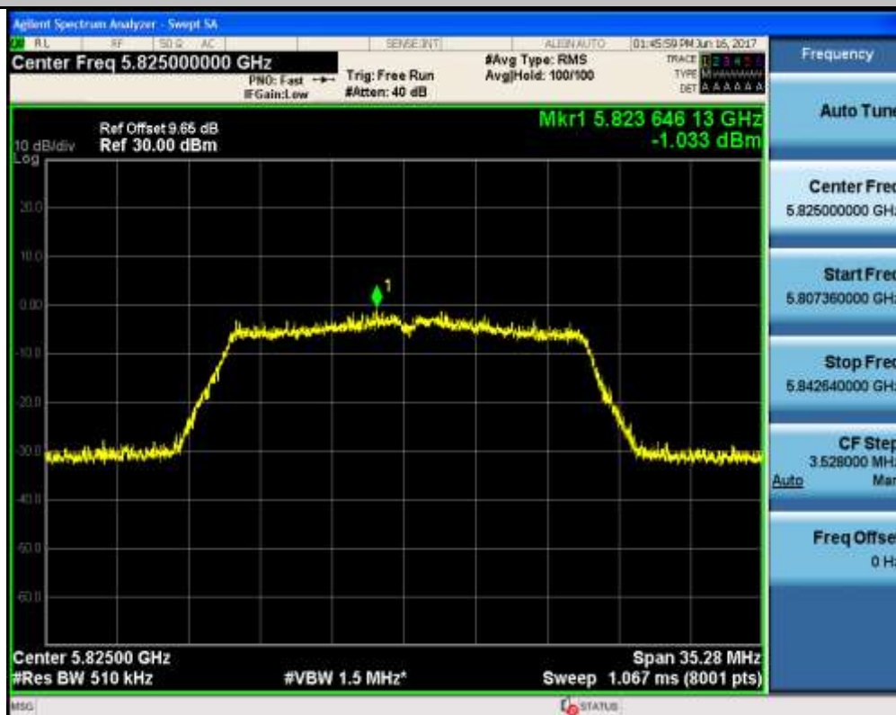
Maximum Conduct Output Power_TNVN_11AC40_5190_Ant1
