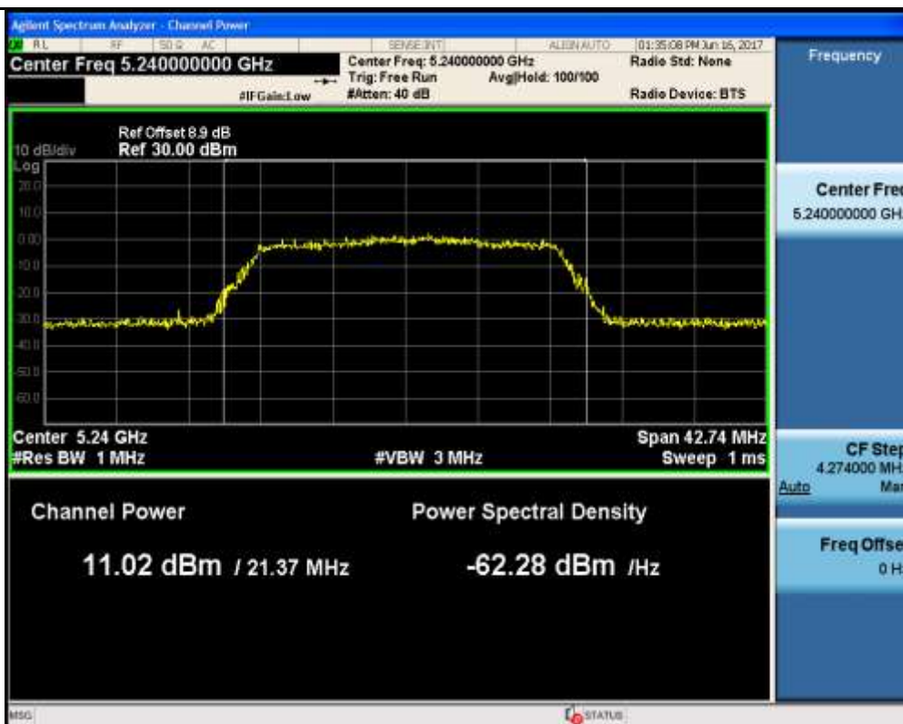
Maximum Conduct Output Power_11AC20_5745_Ant1
