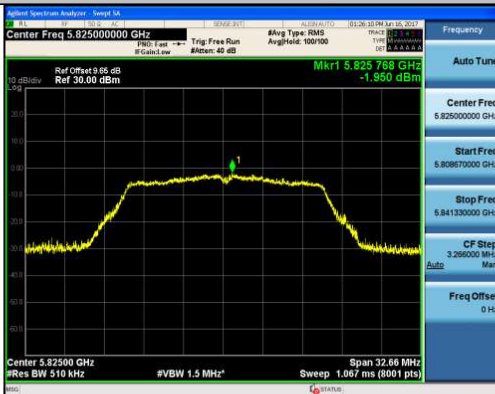
Maximum Conduct Output Power_TNVN_11AC20_5180_Ant1
