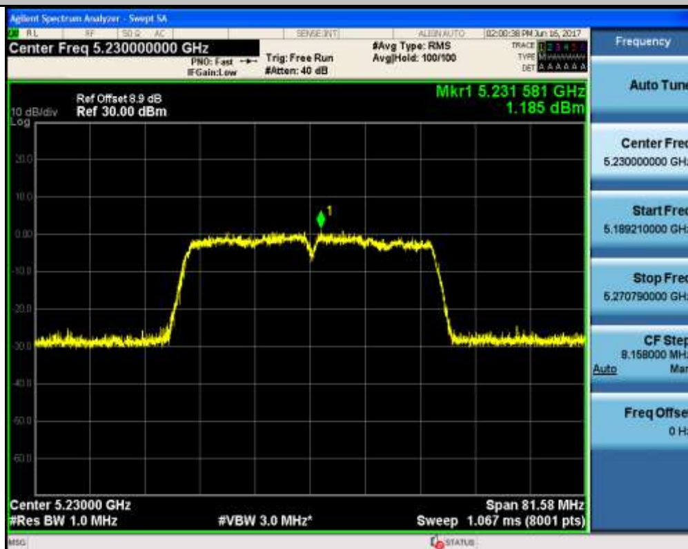
Maximum Conduct Output Power_TNVN_11AC40_5755_Ant1
