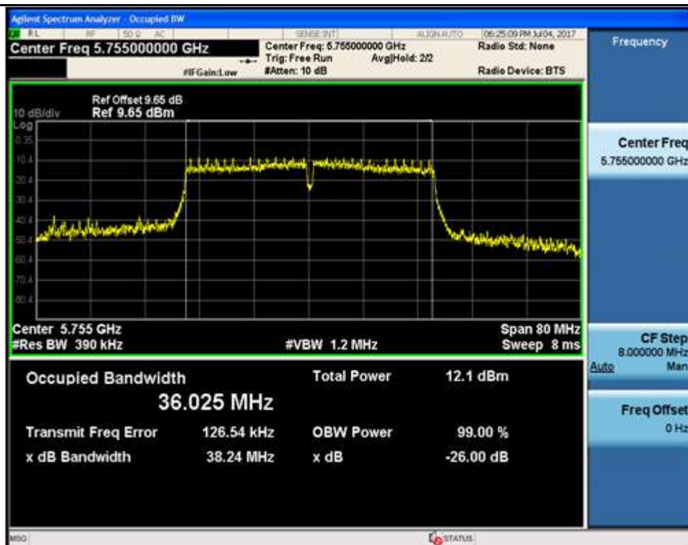
Emission Bandwidth Measurement_11N40_5795_Ant1
