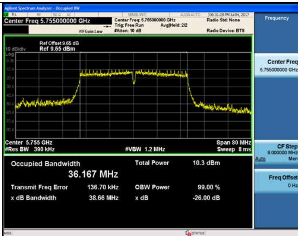
Emission Bandwidth Measurement_11AC40_5795_Ant1
