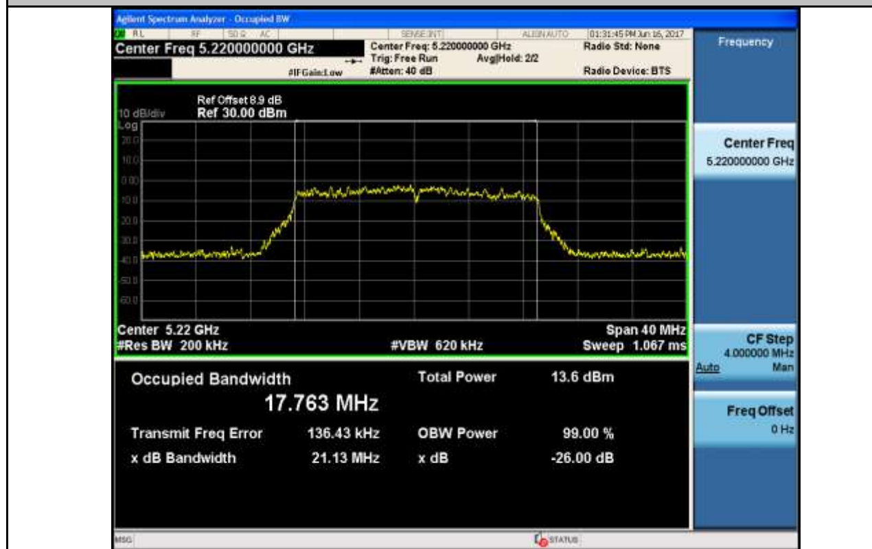
Emission Bandwidth Measurement_11AC20_5240_Ant1
