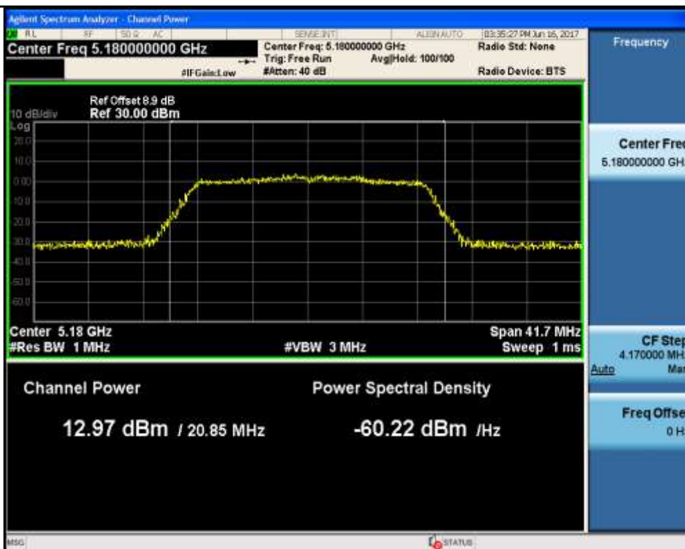
Maximum Conduct Output Power_11N20_5220_Ant1
