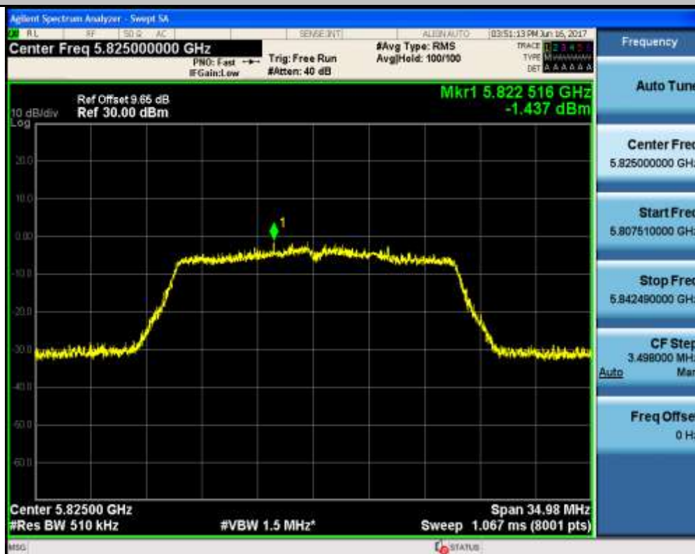
Maximum Conduct Output Power_TNVN_11N40_5190_Ant1
