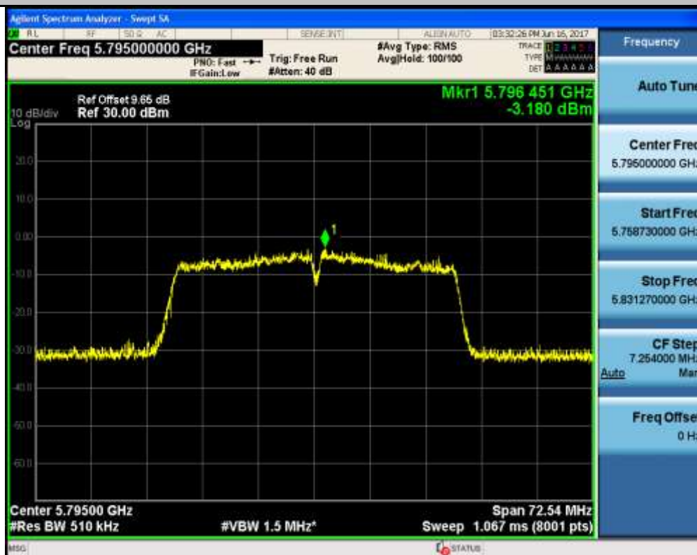
Maximum Conduct Output Power_TNVN_11N20_5180_Ant1
