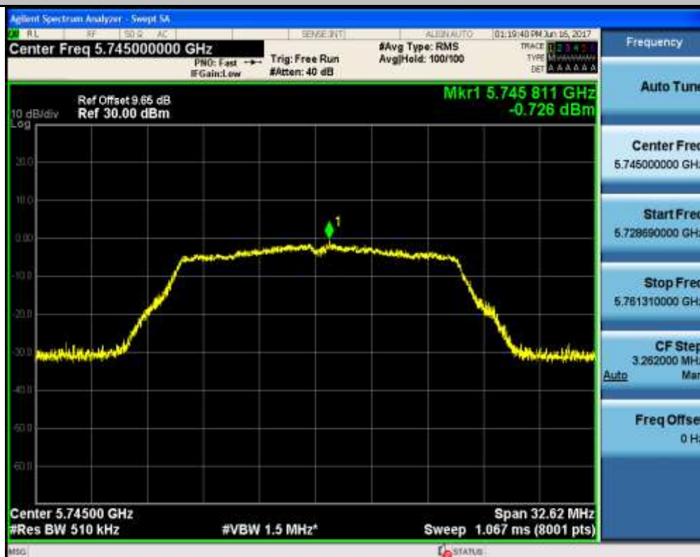
Maximum Conduct Output Power_TNVN_11A_5785_Ant1
