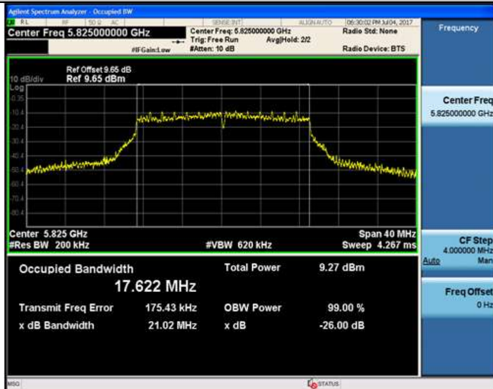
Emission Bandwidth Measurement_11AC40_5190_Ant1
