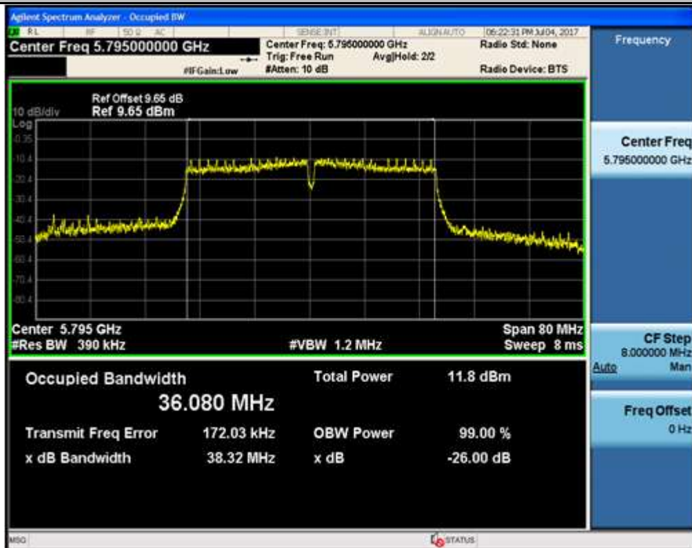
Emission Bandwidth Measurement_11AC80_5210_Ant1
