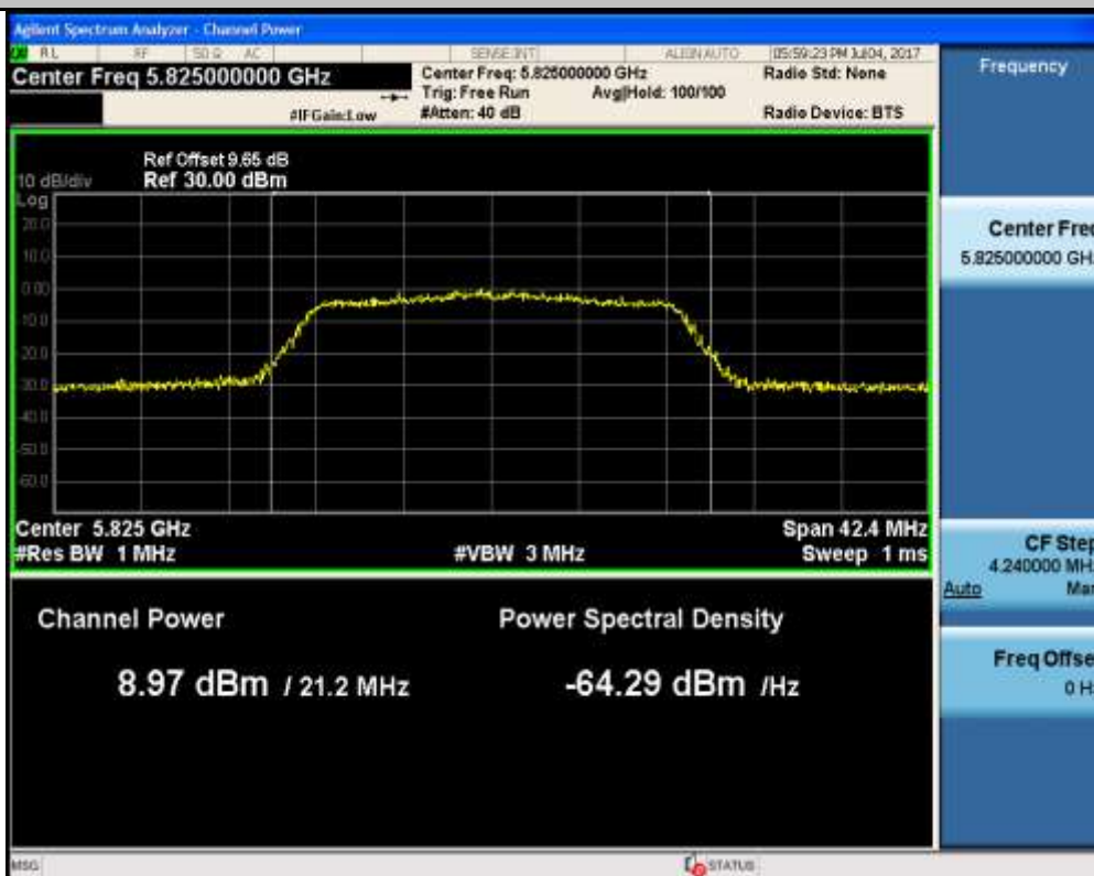
Maximum Conduct Output Power_11N40_5190_Ant1
