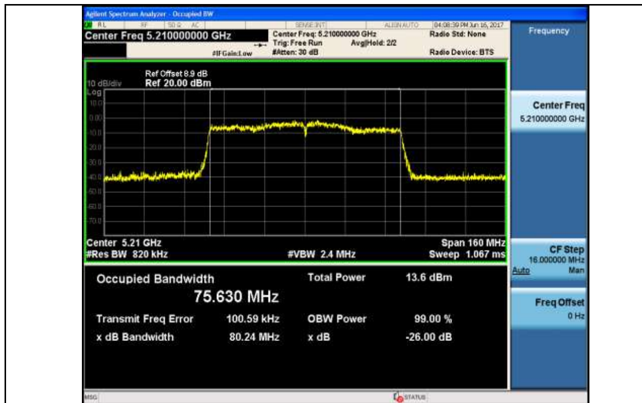
Emission Bandwidth Measurement_11AC80_5775_Ant1
