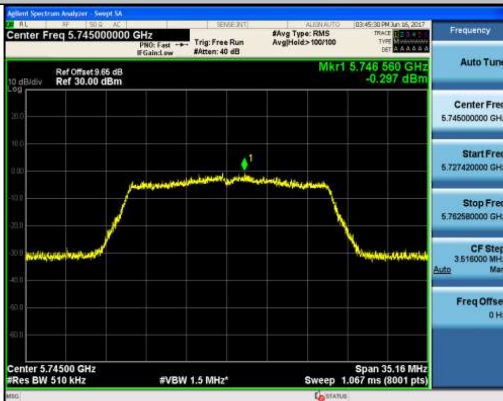
Maximum Conduct Output Power_TNVN_11N20_5785_Ant1
