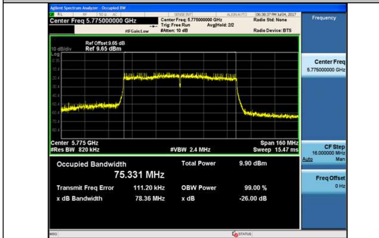
Emission Bandwidth Measurement_11AC80_5775_Ant1
