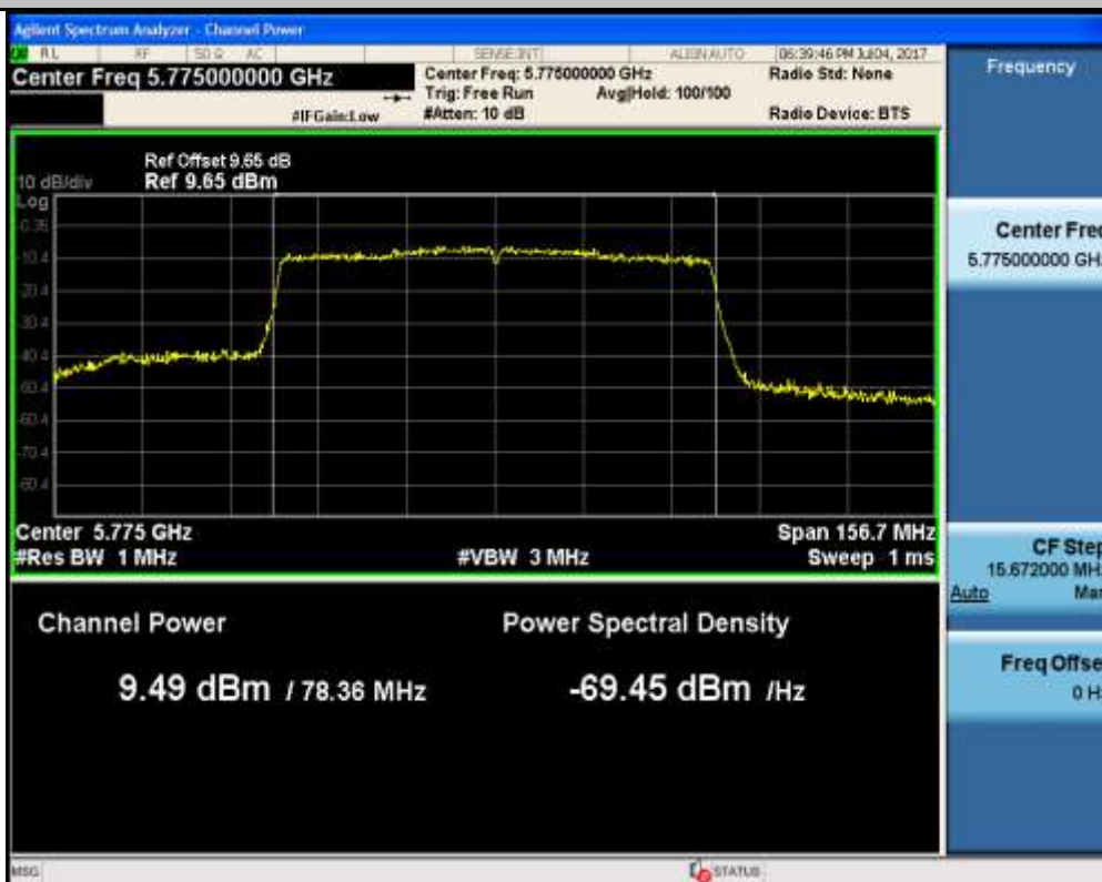
Maximum Conduct Output Power_11AC80_5775_Ant1
