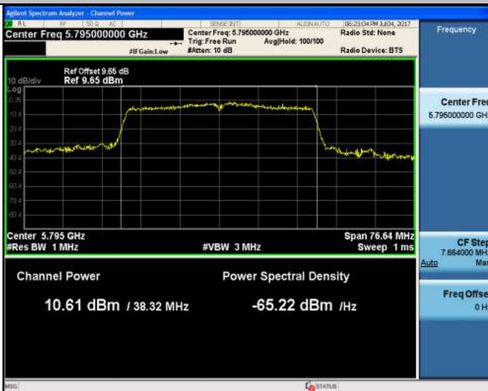
Maximum Conduct Output Power_11AC80_5210_Ant1
