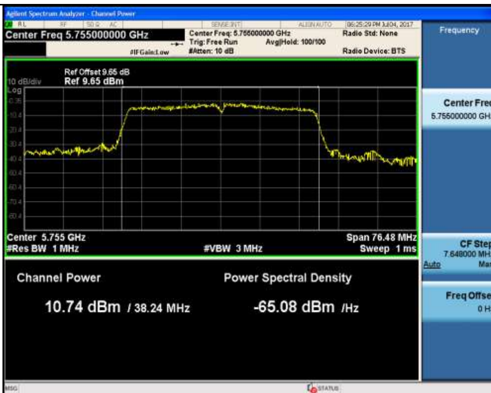
Maximum Conduct Output Power_11N40_5795_Ant1
