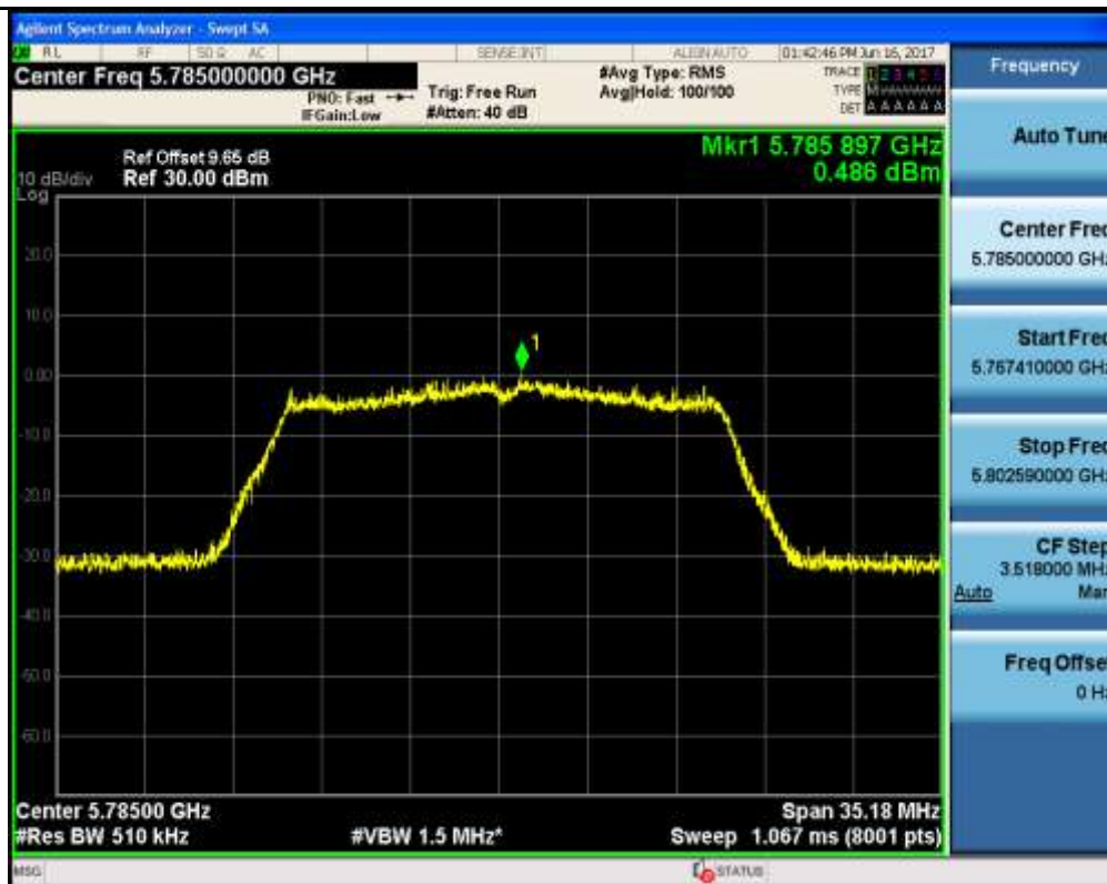
Maximum Conduct Output Power_TNVN_11AC20_5825_Ant1
