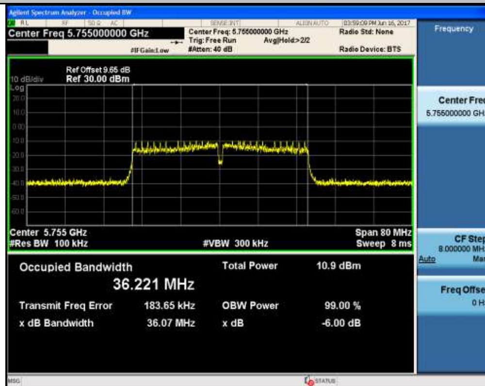
Emission Bandwidth Measurement_11N40_5795_Ant1
