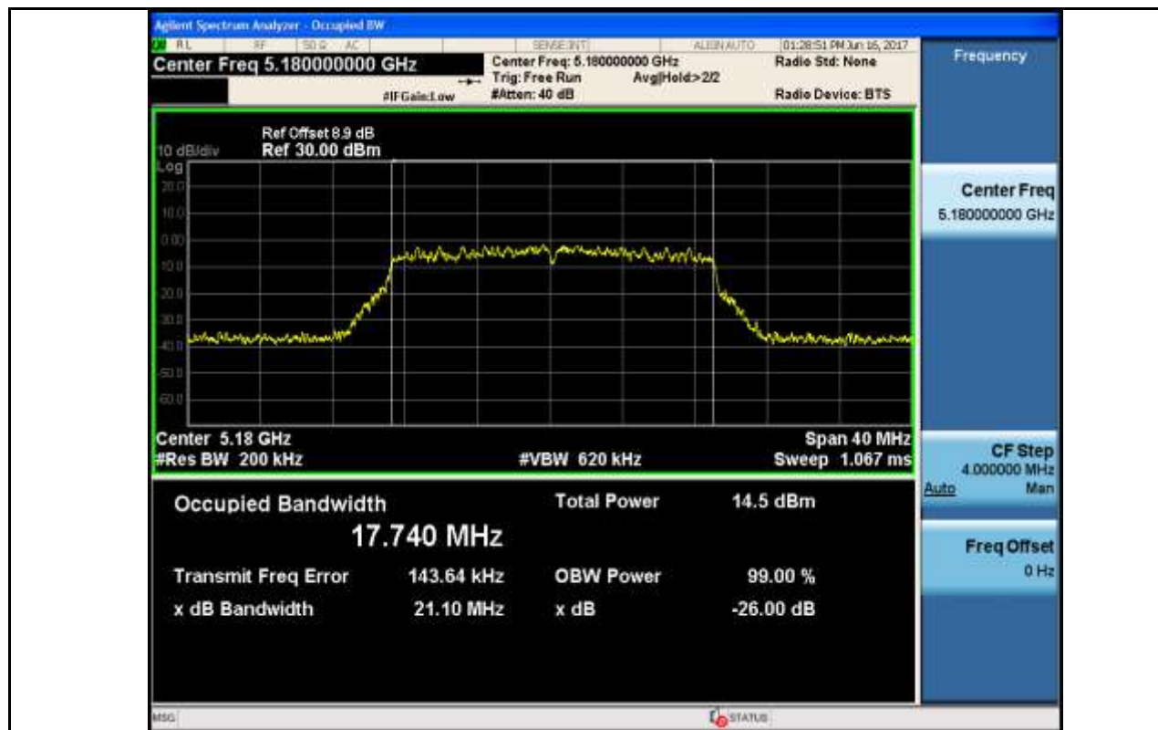
Emission Bandwidth Measurement_11AC20_5220_Ant1
