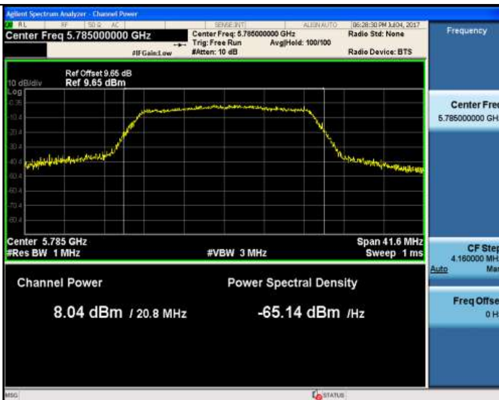
Maximum Conduct Output Power_11AC20_5825_Ant1
