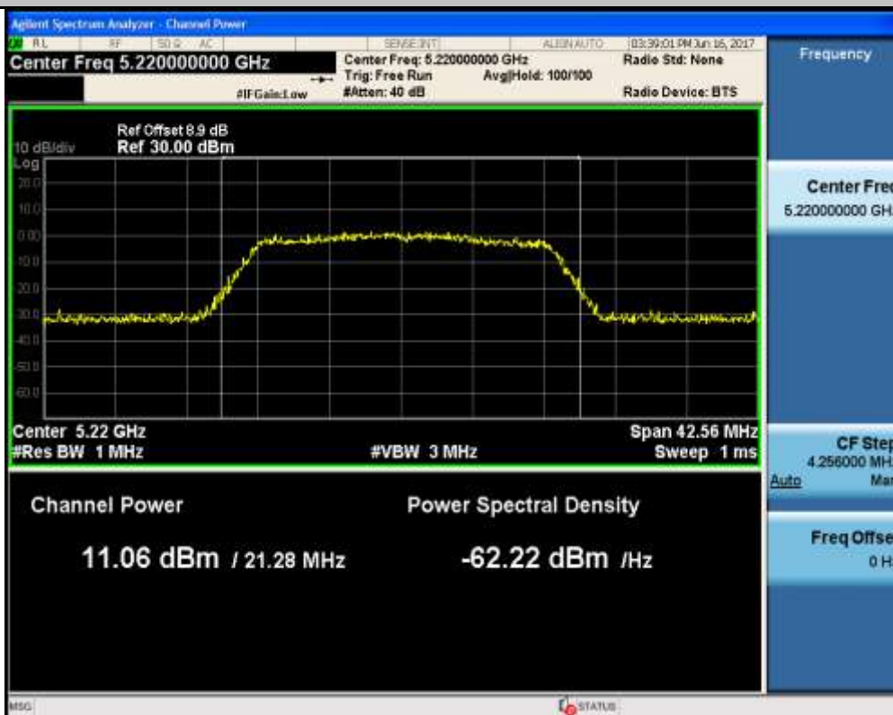
Maximum Conduct Output Power_11N20_5240_Ant1
