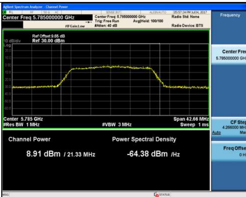
Maximum Conduct Output Power_11N20_5825_Ant1
