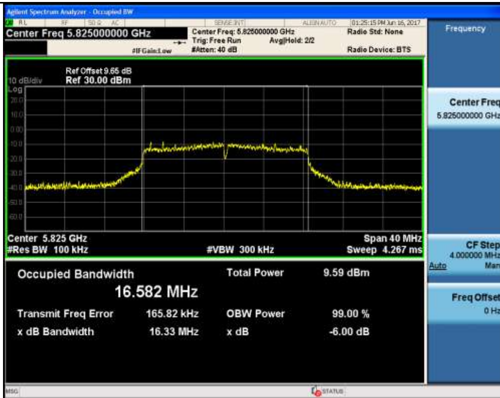
Emission Bandwidth Measurement_11AC20_5745_Ant1
