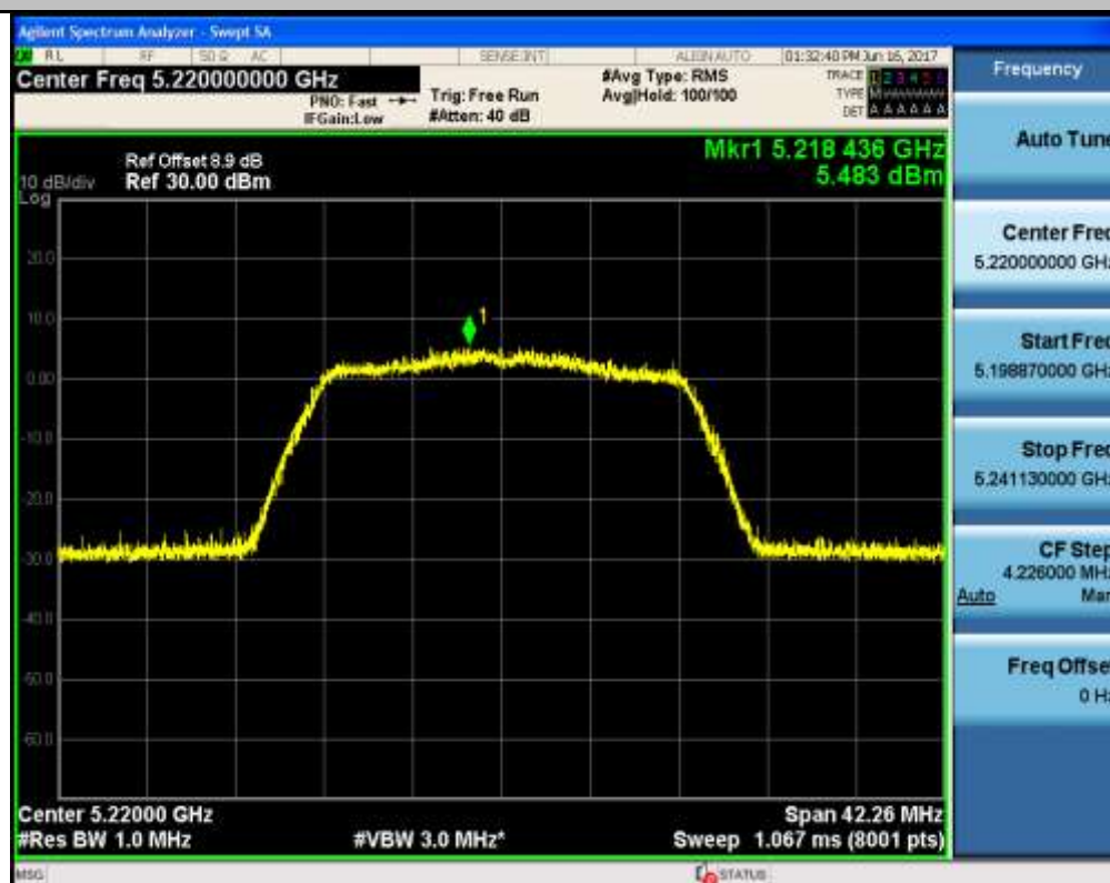
Maximum Conduct Output Power_TNVN_11AC20_5240_Ant1
