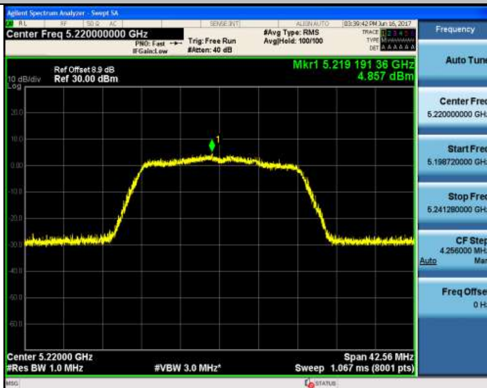
Maximum Conduct Output Power_TNVN_11N20_5240_Ant1
