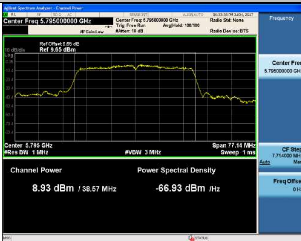
Maximum Conduct Output Power_11N20_5180_Ant1
