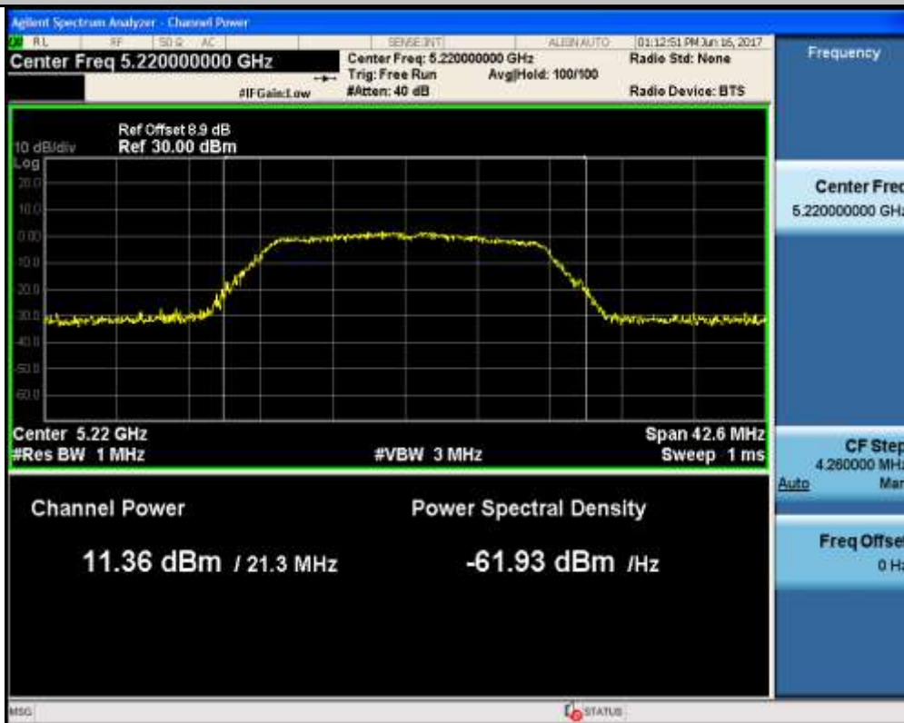
Maximum Conduct Output Power_11A_5240_Ant1
