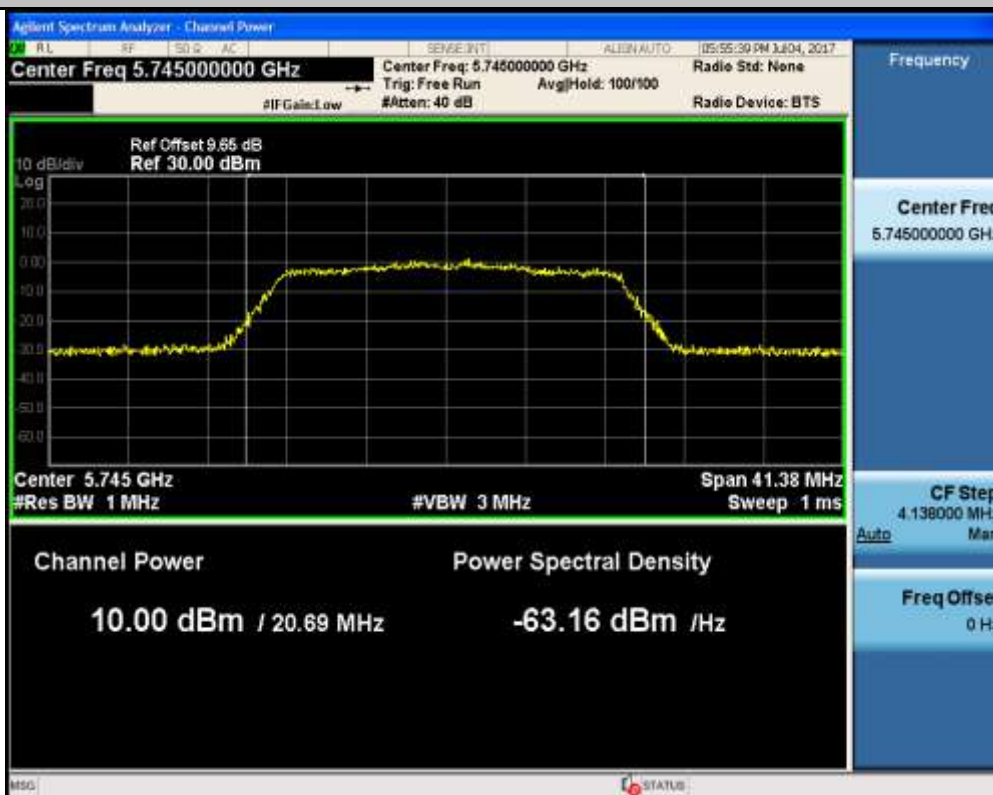
Maximum Conduct Output Power_11N20_5785_Ant1
