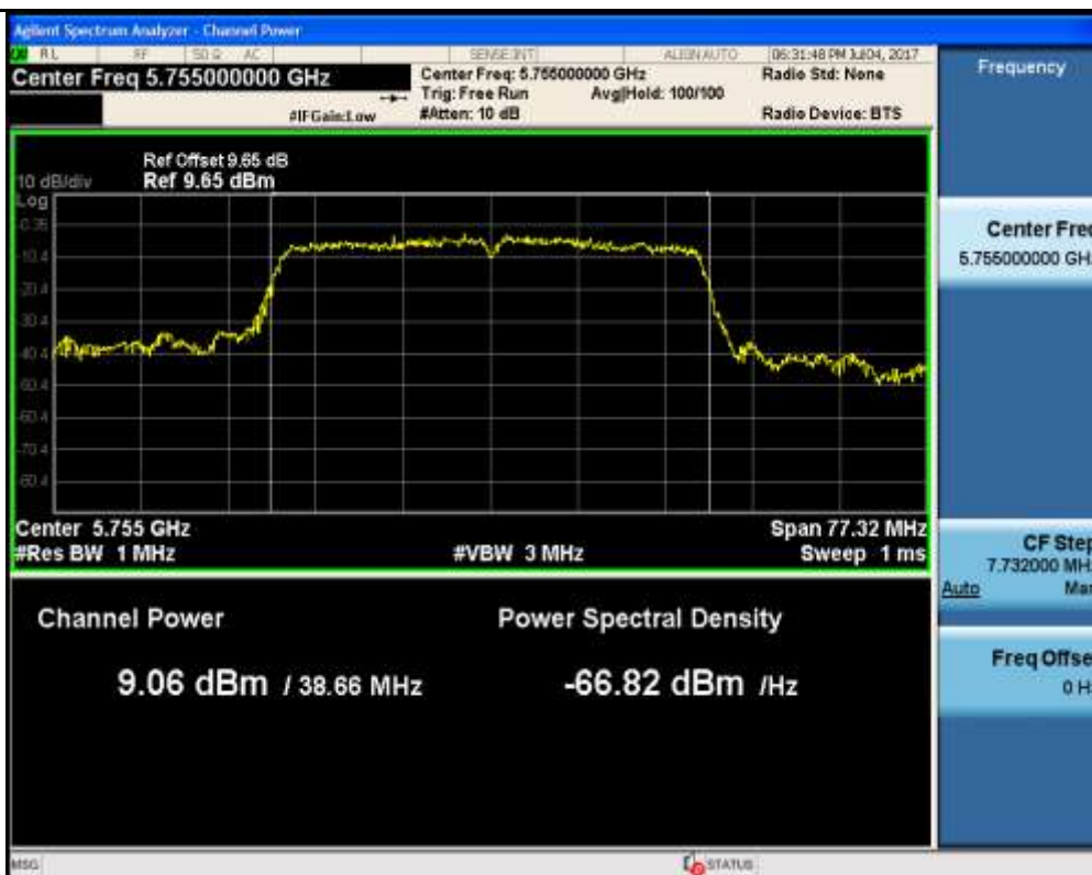
Maximum Conduct Output Power_11AC40_5795_Ant1
